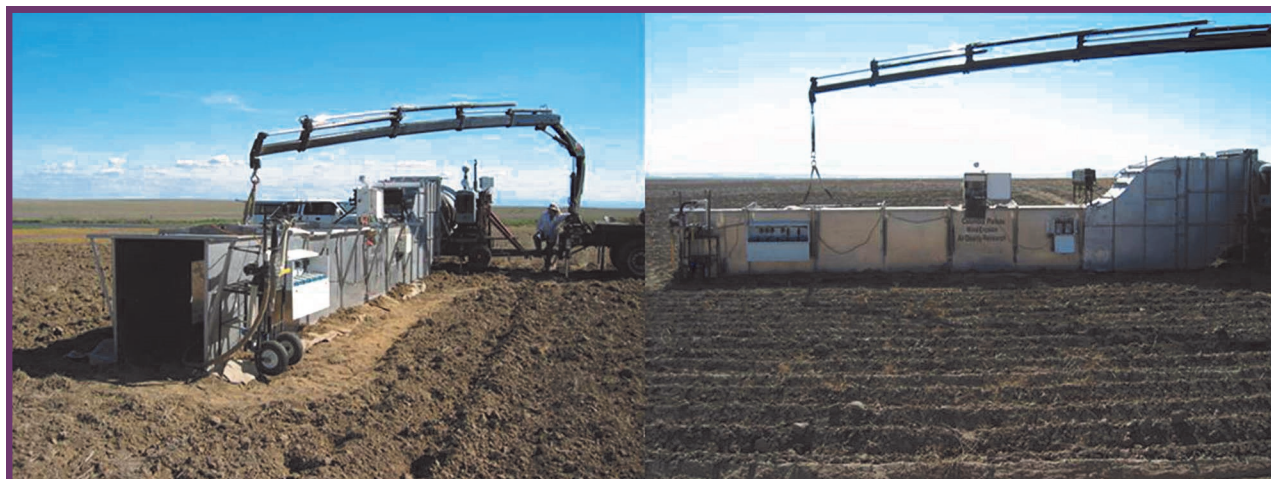
Wind erosion potential from summer fallow tillage treatments in the Horse Heaven Hills using a portable wind tunnel. The left image is traditional-tillage fallow after primary spring tillage at the eastern site and the right image is undercutter-tillage fallow taken after planting winter wheat at the western site.
