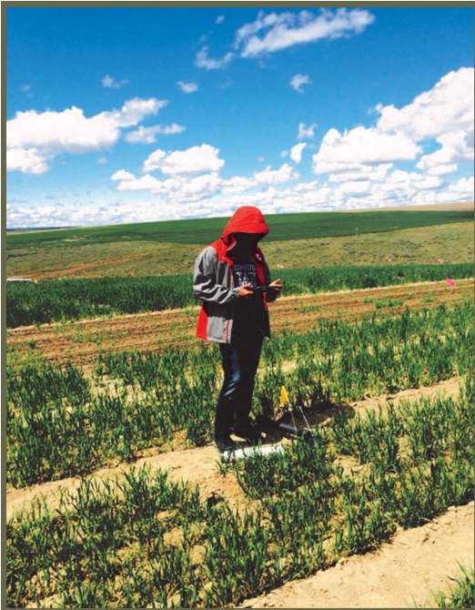
Raul Arroyo from the Sanguinet lab acquiring a 360 scan window of a minirhizotron tube using the CI-600 root scanner in a wheat plot at the Lind Dryland Research Station.
