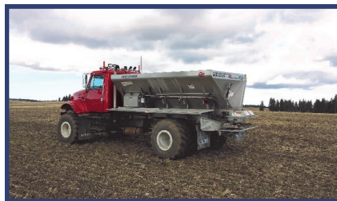
Figure 1. Lime was applied using a two-paddle distributor mounted on a "floater" truck.
