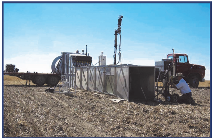
Figure 1. Portable wind tunnel used to assess the wind erosion potential of soils amended with biosolids at Lind, Washington.
