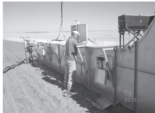
Fig. 1. A portable wind tunnel was used to measure soil sediment flux and PM 10 emissions, shown here at the Ron Jirava farm near Ritzville.
