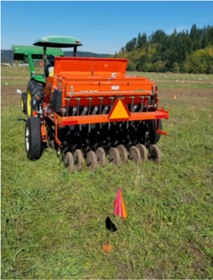
Planting pasture with Pierce CD No-Till drill, September 26, 2018
