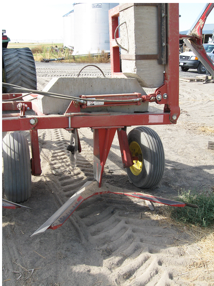
Figure 4. An undercutter like this can be used to incorporate broadcast mustard seed while also killing weeds.
