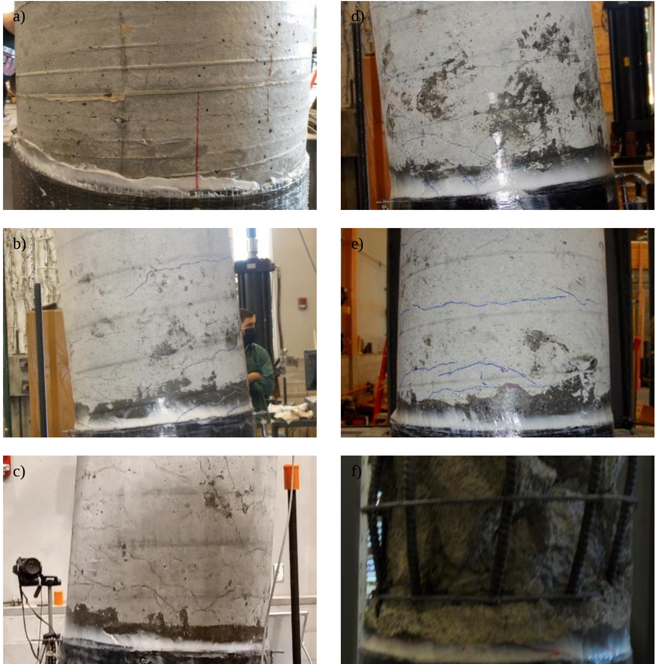
Figure 3.23. Concrete Damage Above Jacket at 20\delta/\delta_y (at 15\delta/\delta_y for C(CFRP)-4.0-#7(1.3)-0.15) for: a) C(CFRP)-4.0-#7(1.3)-0.05, b) C(CFRP)-4.0-#5(1.4)-0.05, c) C(CFRP)-4.0-#7(2.7)-0.05, d) C(CFRP)-4.0-#7(1.3)-0.05-EQ, e) C(CFRP)-4.0-#7(1.3)-0.05-2X, and f) C(CFRP)-4.0-#7(1.3)-0.15
