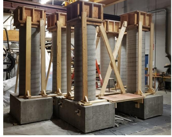
Figure 3.6: Construction: a) Bracing for Column Concrete Pour, and b) Bracing for Top Block Concrete Pour
