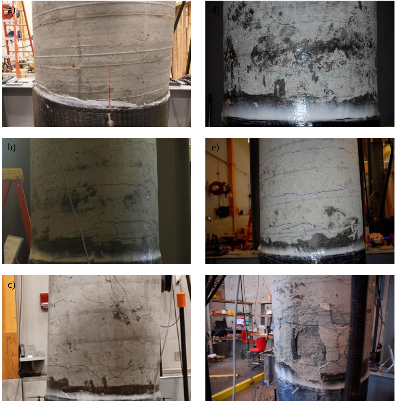
Figure 3.21. Concrete Damage Above Jacket at 15\delta/\delta_y for: a) C(CFRP)-4.0-#7(1.3)-0.05, b) C(CFRP)-4.0-#5(1.4)-0.05, c) C(CFRP)-4.0-#7(2.7)-0.05, d) C(CFRP)-4.0-#7(1.3)-0.05-EQ, e) C(CFRP)-4.0-#7(1.3)-0.05-2X, and f) C(CFRP)-4.0-#7(1.3)-0.15
