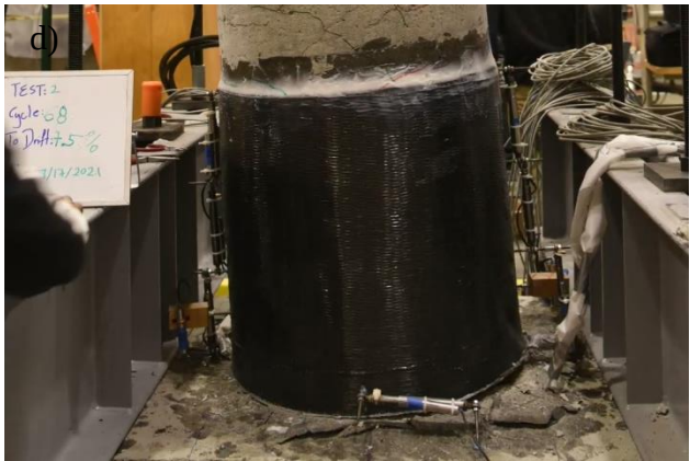
Figure 3.22. Concrete Damage at Base at 20\delta/\delta_y (at 15\delta/\delta_y for C(CFRP)-4.0-#7(1.3)-0.15) for: a) C(CFRP)-4.0-#7(1.3)-0.05, b) C(CFRP)-4.0-#5(1.4)-0.05, c) C(CFRP)-4.0-#7(2.7)-0.05, d) C(CFRP)-4.0-#7(1.3)-0.05-EQ, e) C(CFRP)-4.0-#7(1.3)-0.05-2X, and f) C(CFRP)-4.0-#7(1.3)-0.15
