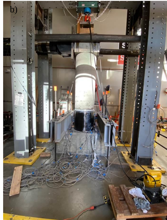
Figure 3.8: Test Set-up, \frac{P_d}{A_g f'_c} = 0.05 : a) Schematic, b) Photo
