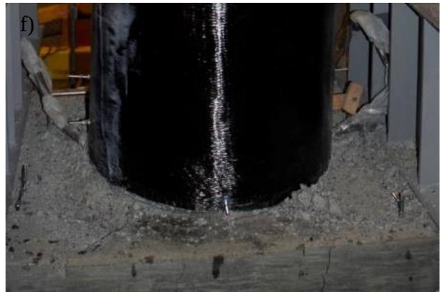
Figure 3.22. Concrete Damage at Base at 20\delta/\delta_y (at 15\delta/\delta_y for C(CFRP)-4.0-#7(1.3)-0.15) for: a) C(CFRP)-4.0-#7(1.3)-0.05, b) C(CFRP)-4.0-#5(1.4)-0.05, c) C(CFRP)-4.0-#7(2.7)-0.05, d) C(CFRP)-4.0-#7(1.3)-0.05-EQ, e) C(CFRP)-4.0-#7(1.3)-0.05-2X, and f) C(CFRP)-4.0-#7(1.3)-0.15
