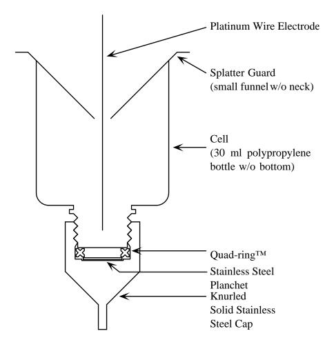
Fig. 1. Electrolytic cell.
