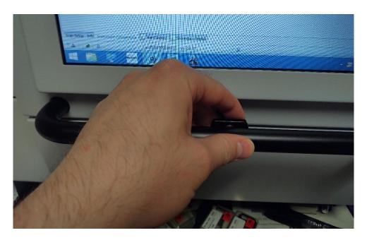
6.41 The door will slide up allowing for the removal of the sample. Pull down on the sample holder latch, which will cause the sample to lower. Remove the sample after it has lowered.
