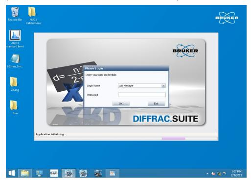
6.9 After clicking OK, the software will say that the Measurement Server is running, this software is necessary for the instrument to talk to the data collection software.
