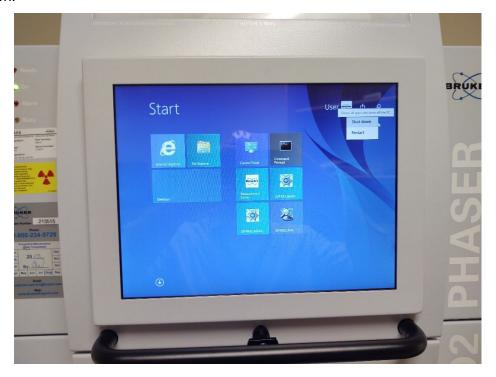
8.2 Wait until you see the following message before turning off the power switch on the back of the instrument (see step 6.3 for power switch location).
