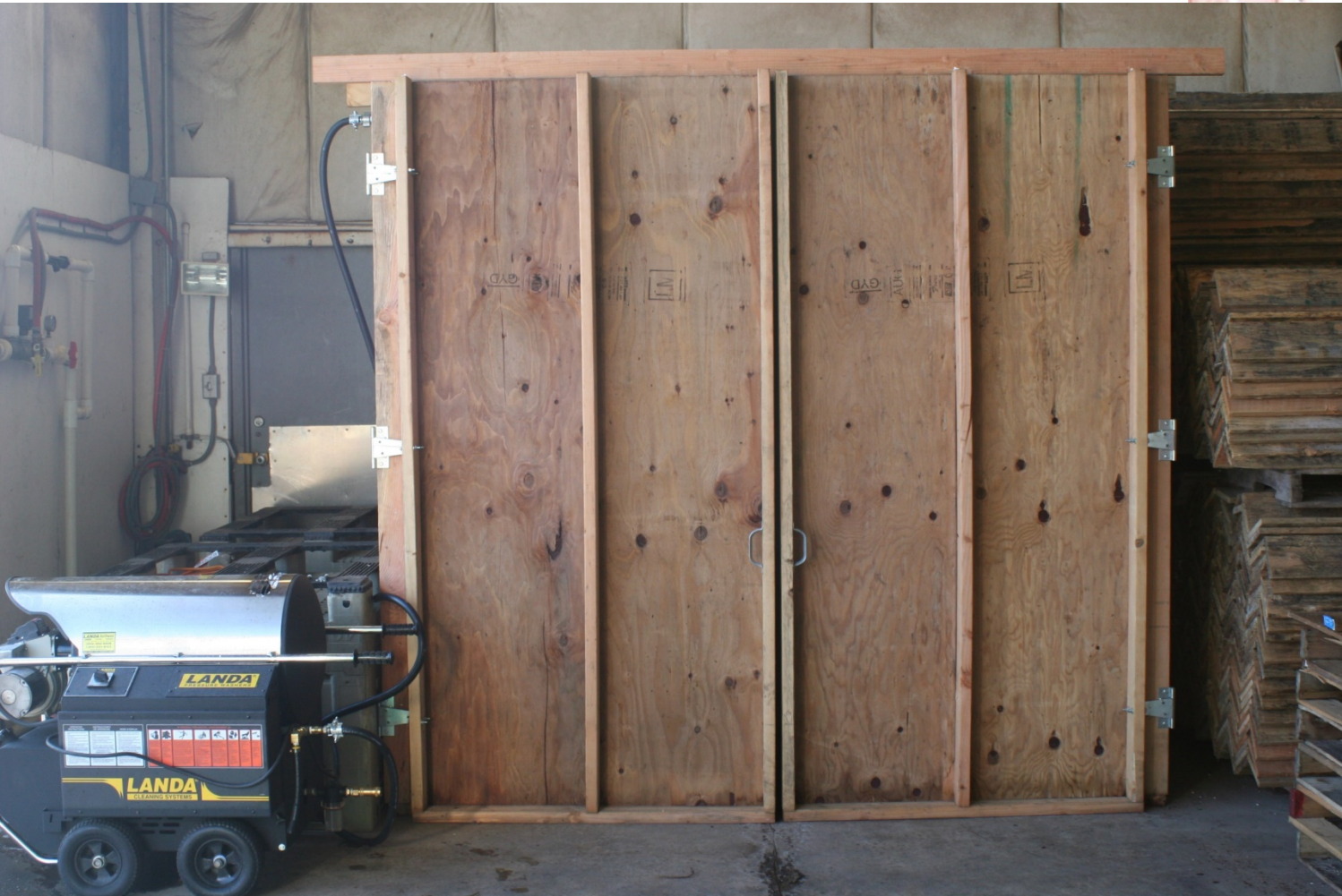
This steam cabinet was built on a relatively low budget by a nursery in OR
