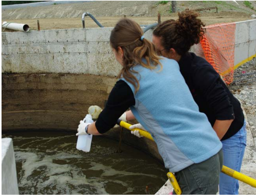
Figure 13. Sampling incoming manure and pre-consumer food-wastes at the receiving tank
