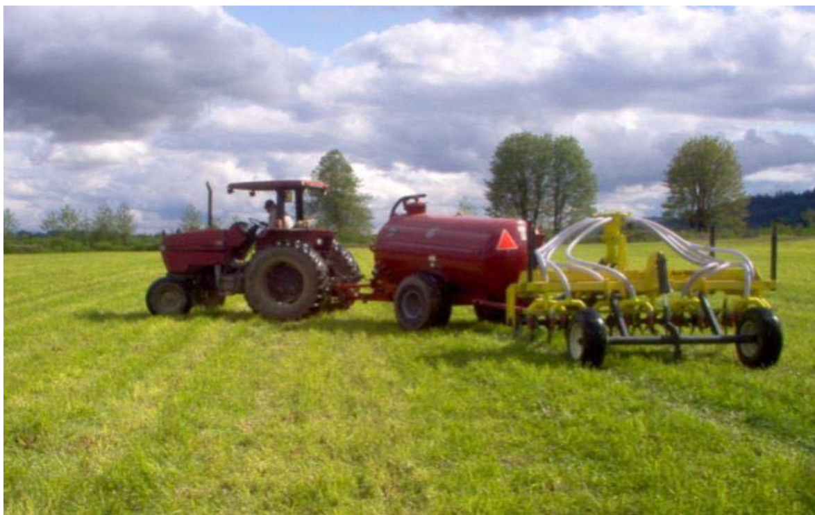
Figure 36. Manure application tank with Aerway® TM applicator.
