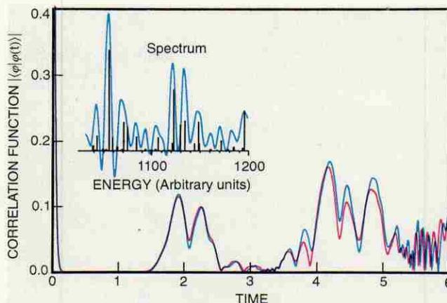
**Autocorrelation function**  $C(t) = \langle \phi | \phi(t) \rangle$  for the system shown in figure 7, computed using quantum and semiclassical evolution (red and blue curves, respectively). Inset shows the spectrum obtained by taking the Fourier transform of  $C(t)$  (blue) and the numerically determined exact spectrum. (Adapted from ref. 24.) **Figure 8**
