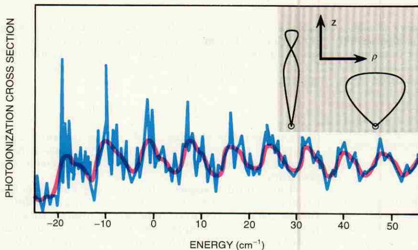
**Photoionization cross section** of a hydrogen atom in a strong magnetic field in the chaotic regime. Medium- and low-resolution spectra (blue and red curves, respectively) clearly exhibit structure, which was ascribed to the returning orbits sketched in the inset. The direction of the magnetic field is along  $z$ . The energy zero is at the energy of ionization. (Adapted from ref. 14.) **Figure 3**
