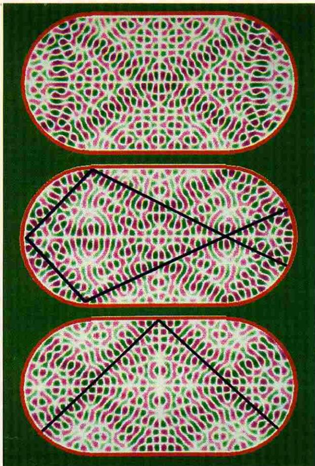
Typical 'scarred' eigenstates of the stadium billiard. These are plots of  $\psi$  for numerically accurate eigenstates. The scars, regions of high amplitude, are generated by periodic orbits, two of which are shown. **Figure 2**
