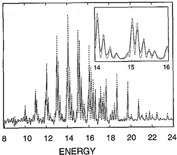
FIG. 5. The spectrum (numerical FFT of the autocorrelation function) of the initial wave packet discussed in the text, comparing the exact quantum result (FFT) and the semiclassical Van Vleck Green's function propagation. A detail is also shown.
