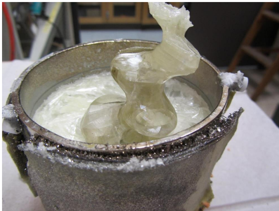
Figure 4.1: \text{Ga}_2\text{O}_3 boule still in the iridium crucible.
