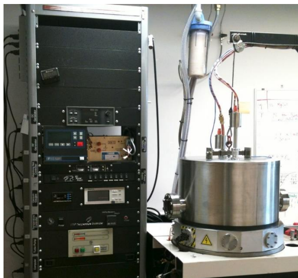
Figure 3.7: Sputtering system in the Bergman lab at University of Idaho.
