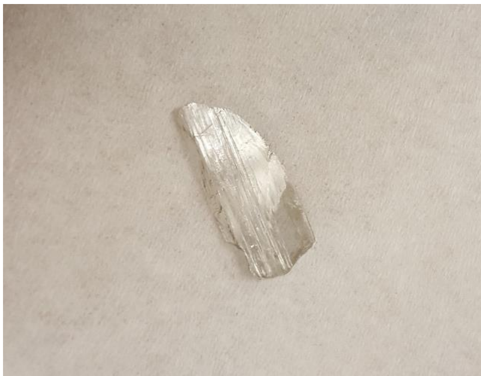
Figure 4.2: Sample crystal of Mg-doped gallium oxide broken from the larger boule
