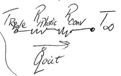
$$\dot{q}_{out} = \frac{T_{R_{Bale}} - T_{\infty}}{R_{plastic} + R_{conv}}$$
