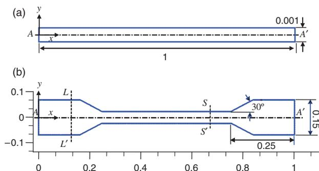
**Fig. 1.** Schematic of 2D microchannel geometries used in the numerical simulation of ampholyte-based IEF. (a) Straight microchannel and (b) contraction-expansion microchannel. All dimensions are in [cm]. In the contraction-expansion microchannel, the widths at the expanded ( $L - L'$ ) and throat ( $S - S'$ ) regions are 1.5 mm and 0.5 mm, respectively.
