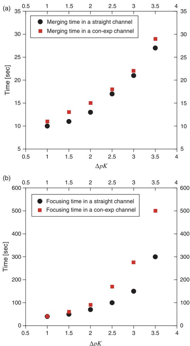
Fig. 5. Comparison of (a) merging time and (b) focusing time for straight and contraction-expansion microchannels.
