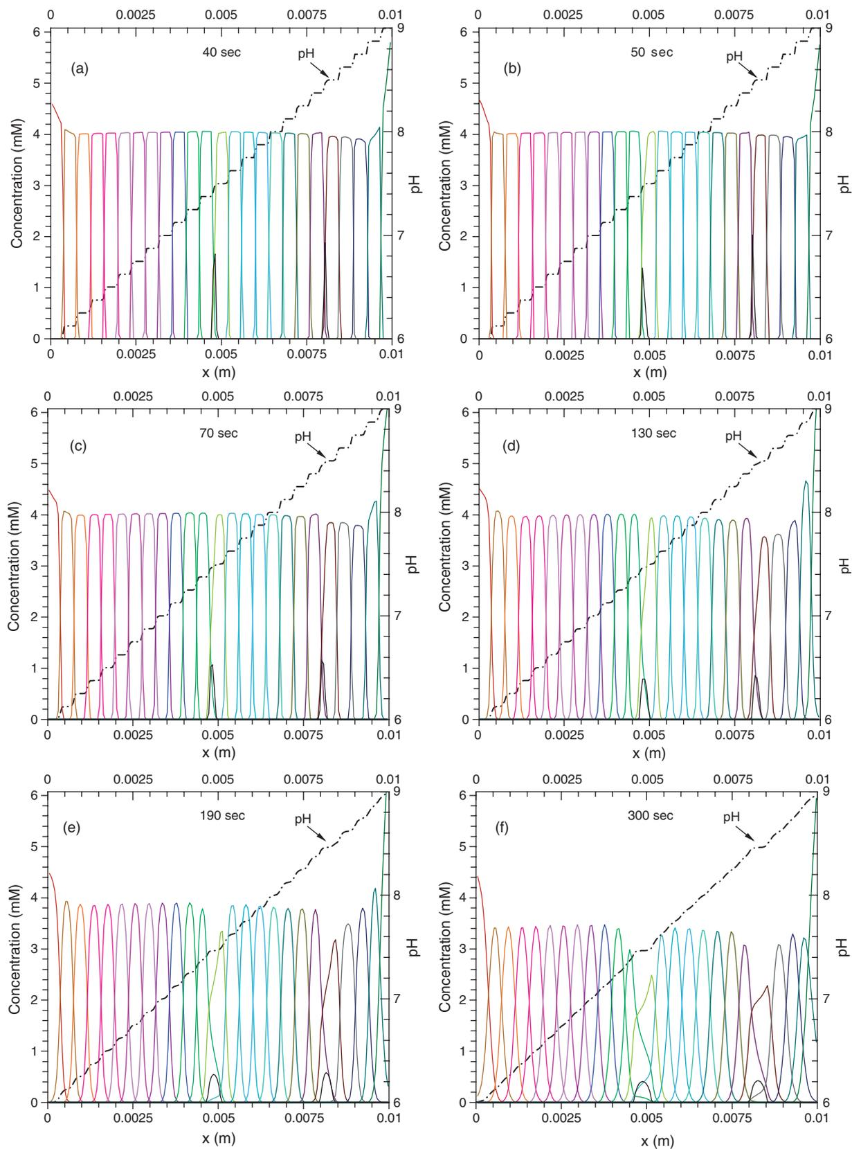
**Fig. 2.** Steady state concentration distribution for ampholytes and proteins in a straight microchannel. (a)  $\Delta pK = 1$ , (b)  $\Delta pK = 1.5$ , (c)  $\Delta pK = 2$ , (d)  $\Delta pK = 2.5$ , (e)  $\Delta pK = 3$ , and (f)  $\Delta pK = 3.5$ . Numerical results are extracted along the channel center line ( $A - A'$ ) of Figure 1(a).
