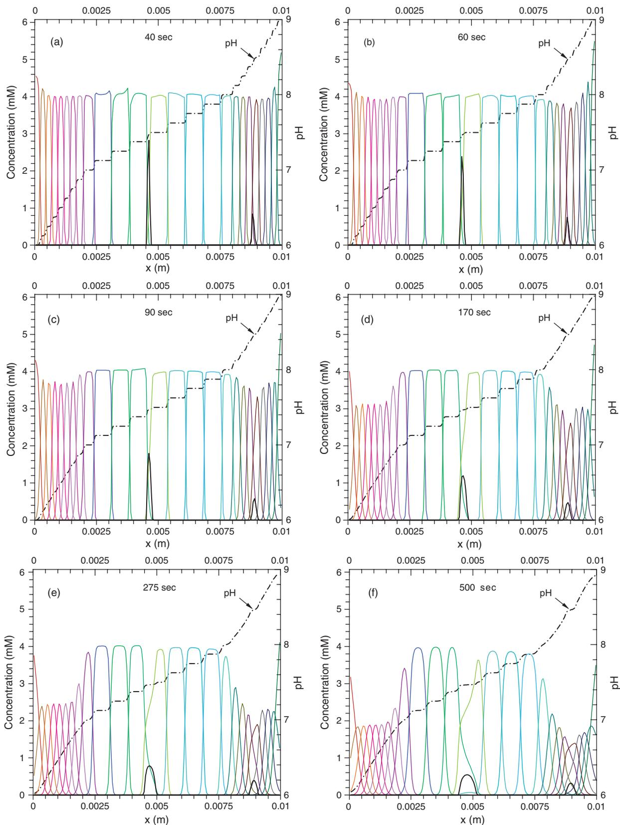
**Fig. 4.** Steady state concentration distribution for ampholytes and proteins in a contraction-expansion microchannel. (a)  $\Delta pK = 1$ , (b)  $\Delta pK = 1.5$ , (c)  $\Delta pK = 2$ , (d)  $\Delta pK = 2.5$ , (e)  $\Delta pK = 3$ , and (f)  $\Delta pK = 3.5$ . Numerical results are extracted along the channel center line ( $A-A'$ ) of Figure 1(b).
