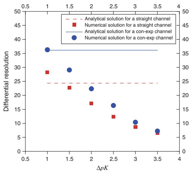
**Fig. 6.** Differential resolution of focused proteins in straight and contraction-expansion microchannels. Eqs. (12) and (15) are used to calculate theoretical and numerical differential resolution, respectively. The numerical differential resolution decreases with increasing  $\Delta pK$ , while the analytical differential resolution remains constant for a particular protein.
