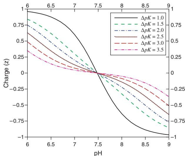
**Fig. 3.** Titration curves of ampholyte #13 ( $pI = 7.50$ ) at different  $\Delta pK$ s. For smaller values of  $\Delta pK$ , the charge gradient is very steep at isoelectric points, which helps in forming rectangular shape tight focused bands of ampholytes.
