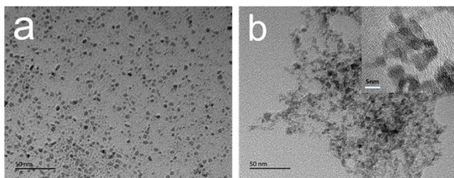
Fig. 3. (a) TEM images of the precursor dissolved in cyclohexane, and (b)  $Gd_2Zr_2O_7$  particles obtained from the precursor calcined at 700 °C for 3 h.
