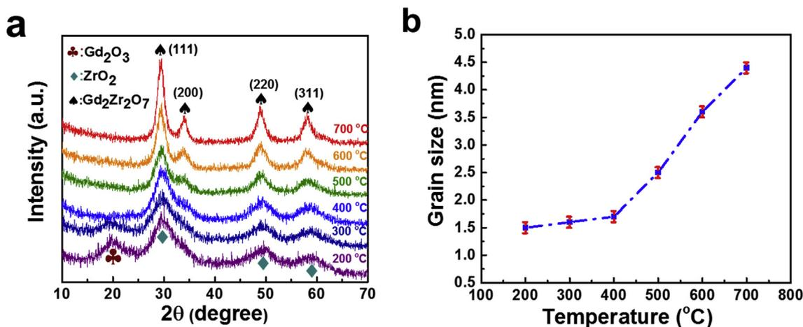
Fig. 2. (a) XRD patterns of the precursor after calcination at 200, 300, 400, 500, 600 and 700 °C for 3 h, and (b) the grain size calculated by Scherrer's formula as a function of calcination temperature.
