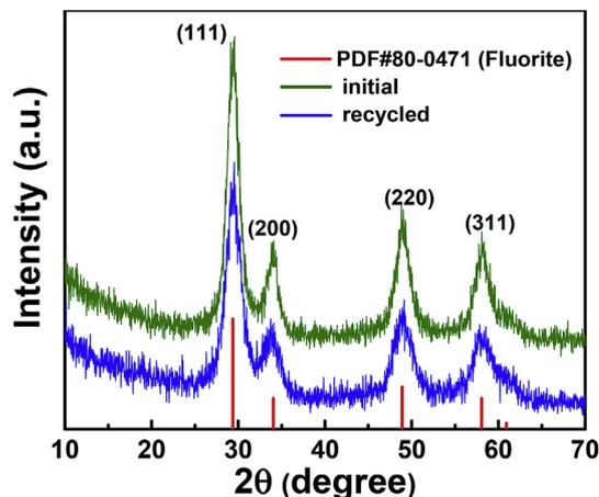
Fig. 4. The XRD patterns of  $Gd_2Zr_2O_7$  nanoparticles synthesized from initial solvent (green) and recycled supernatant solution (blue). (For interpretation of the references to colour in this figure legend, the reader is referred to the Web version of this article.)
