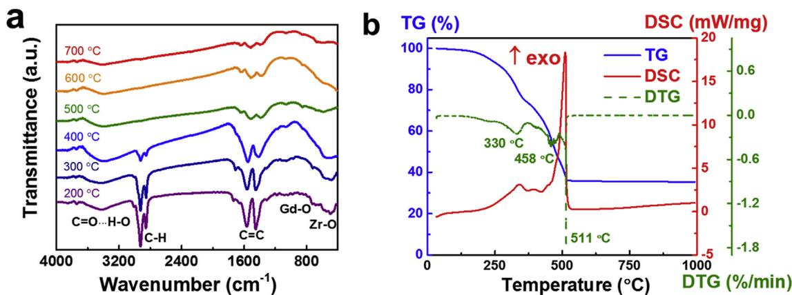
Fig. 1. (a) The FTIR spectra of the precursor after calcination at 200, 300, 400, 500, 600 and 700 °C for 3 h, and (b) the TG-DSC-DTG curve of the precursor calcined in air.
