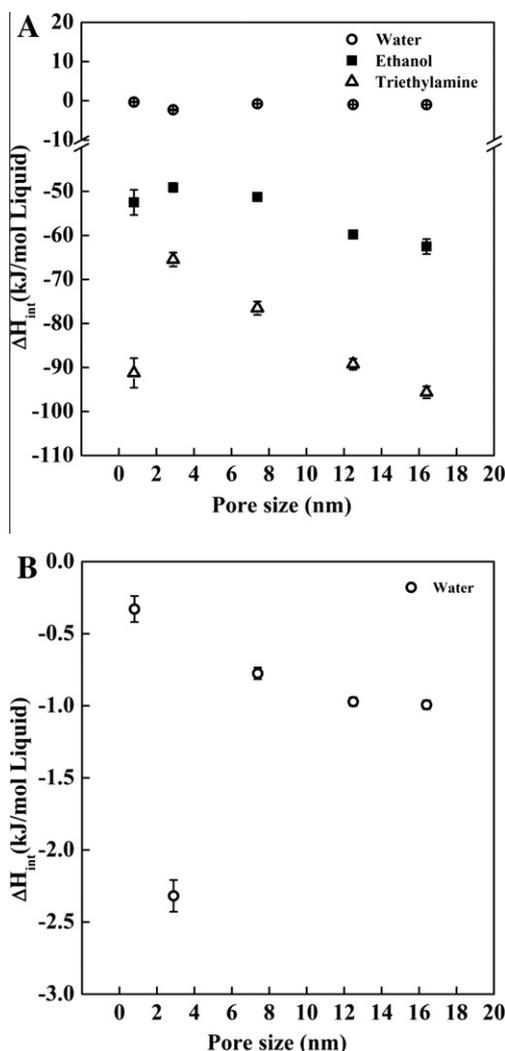
Fig. 6. (a) Enthalpies of interaction for porous silica samples per mole of liquid vs. pore size in water, ethanol and triethylamine. (b) Enthalpies of interaction for porous silica samples per mole of liquid vs. pore size in water.
