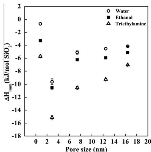
Fig. 3. Enthalpies of immersion for porous silicas per mole of SiO<sub>2</sub> vs. pore size in water, ethanol and triethylamine.
