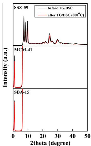
Fig. 1. Powder X-ray diffraction patterns of all porous silica phases in this work (before and after calcination at 800 °C).
