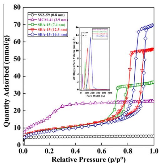
Fig. 2. Nitrogen adsorption/desorption isotherms and pore size distribution curves of all porous silicas used in this work.
