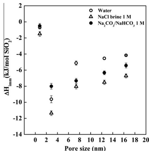
Fig. 4. Enthalpies of immersion for porous silicas per mole of SiO<sub>2</sub> vs. pore size in water, NaCl brine (1 M) and Na<sub>2</sub>CO<sub>3</sub>/NaHCO<sub>3</sub> buffer solution (1 M).
