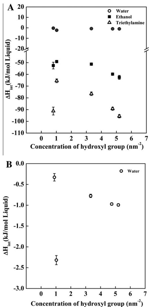
Fig. 7. (a) Enthalpies of interaction for porous silica samples per mole of liquid vs. concentration of hydroxyl group per nm<sup>2</sup> in water, ethanol and triethylamine. (b) Enthalpies of interaction for porous silica samples per mole of liquid vs. concentration of hydroxyl group per nm<sup>2</sup> in water.
