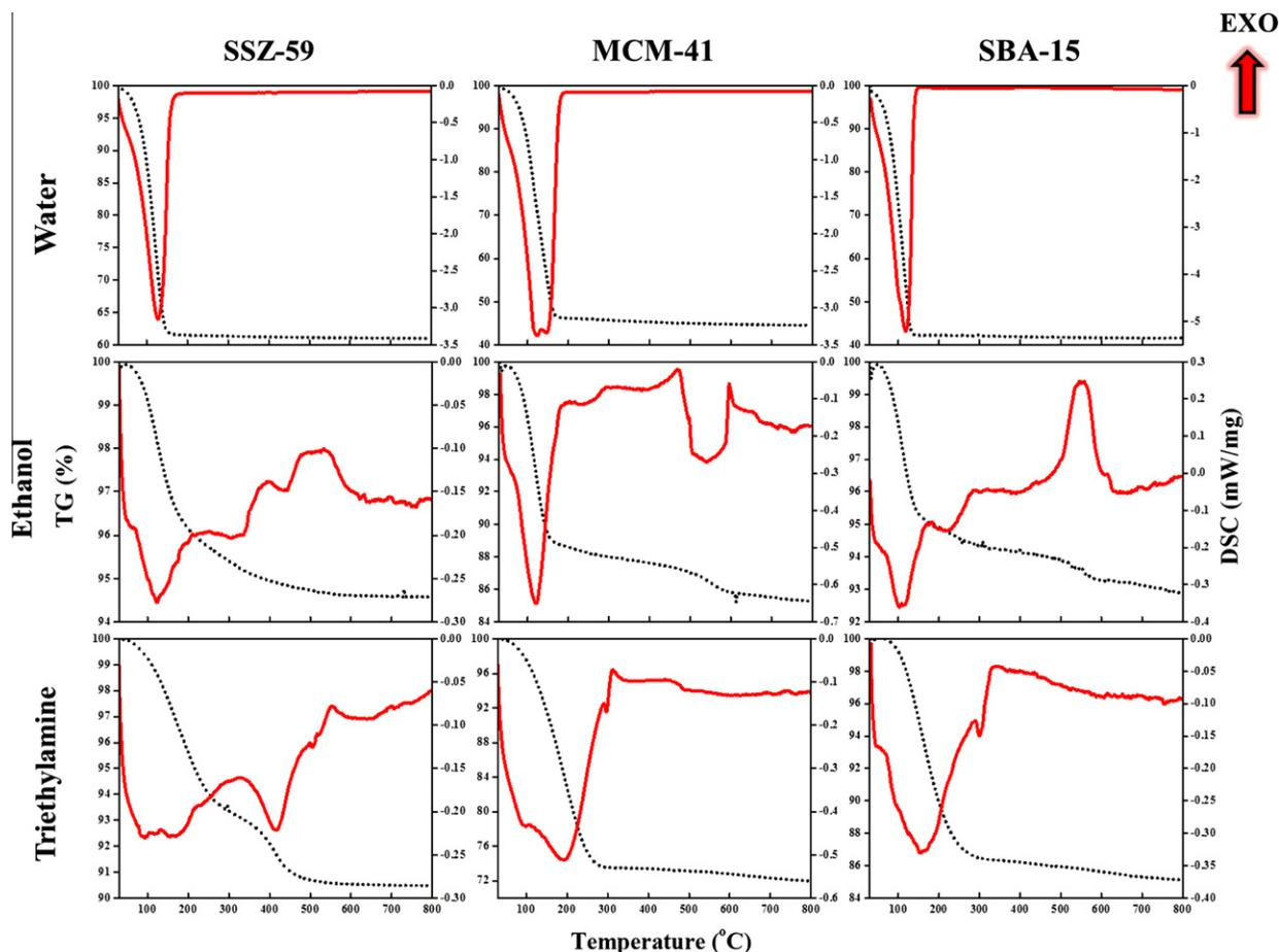
Fig. 5. TG–DSC curves (under argon at 10 °C/min) of SSZ-59, MCM-41 and SBA-15\_3 after immersion calorimetry experiments with water, ethanol and triethylamine.
