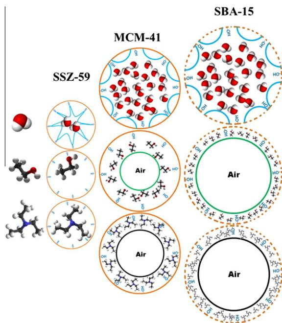
Fig. 8. Proposed structures of water (top), ethanol (middle) and triethylamine (bottom) in pores of SSZ-59 (left), MCM-41 (center) and SBA-15 (right). Dimensions are approximate.
