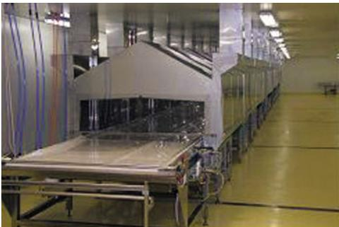
FIG. 1. Model 5 Refractance Window<sup>®</sup> dryer.
