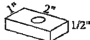
EPDM1 ADHESIVE BACKED RUBBER SPACER (USED AT THE 8mm ROOF ONLY TRIPLEWALL)
