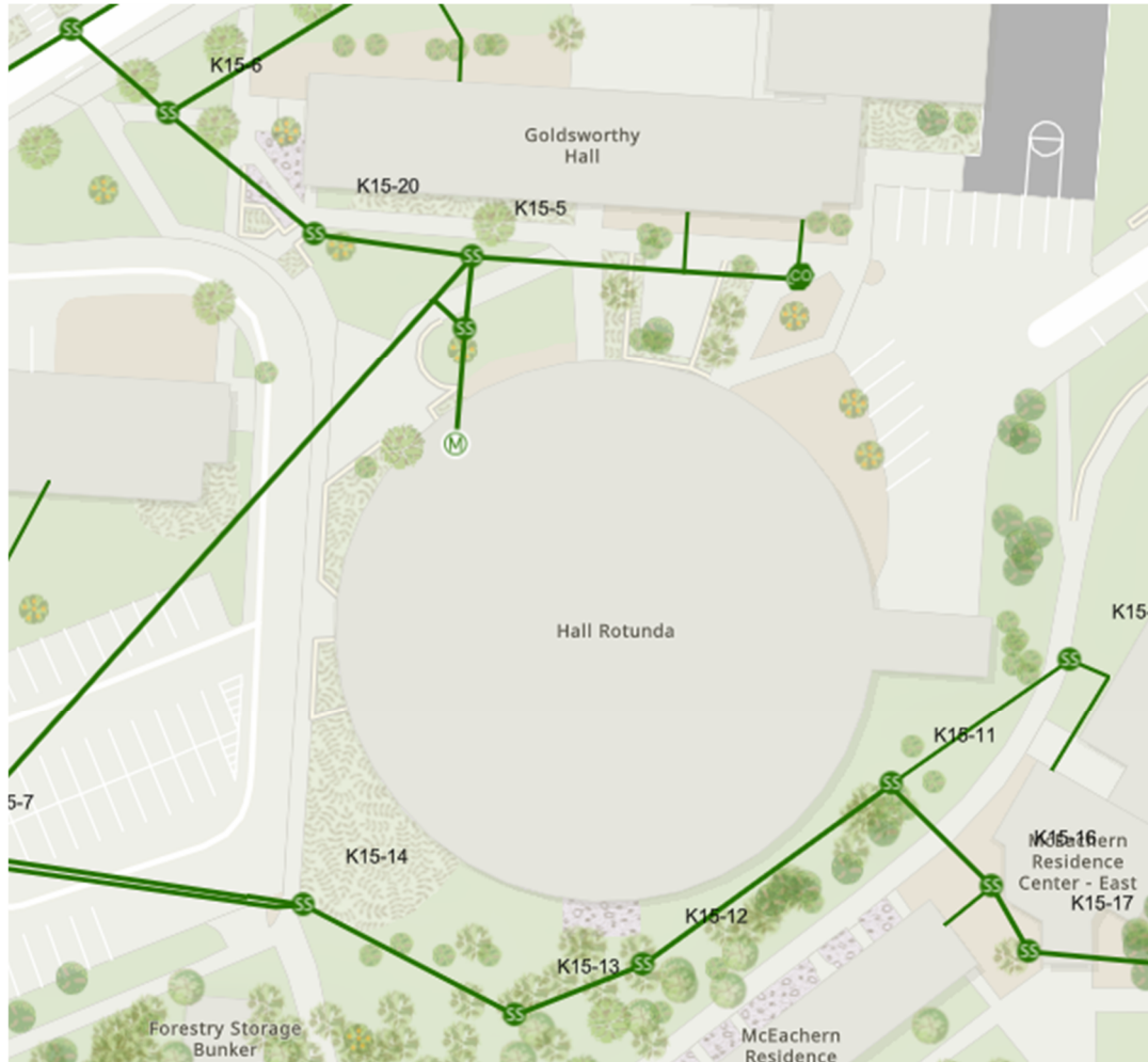
Figure 4 Existing Sewer Mapping
