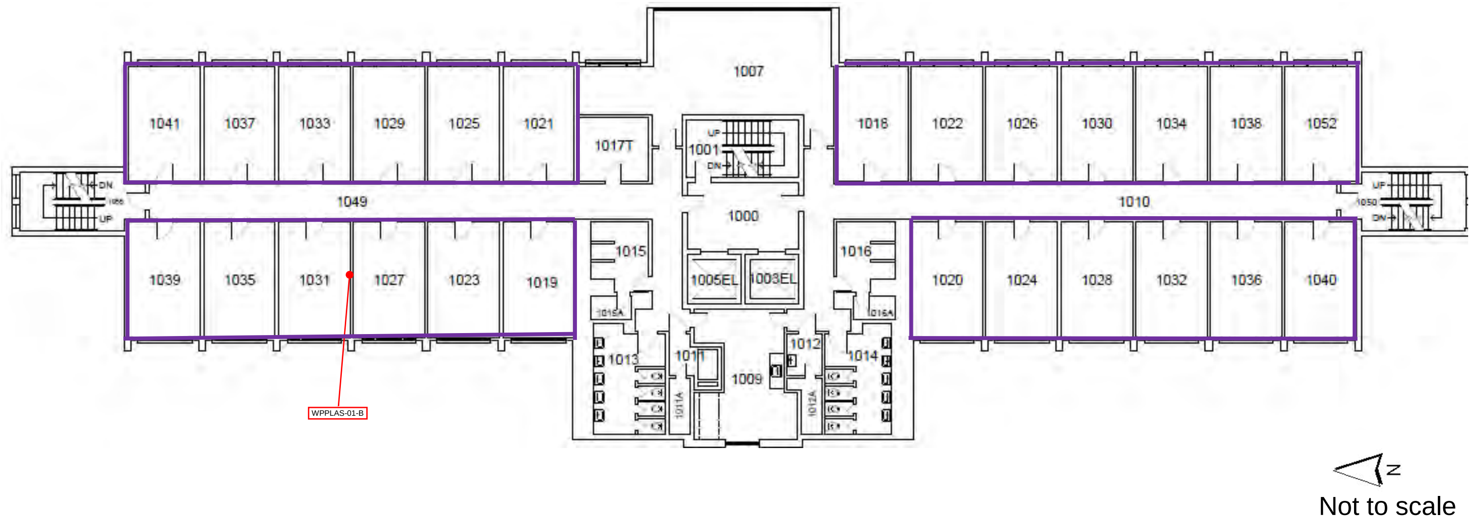
Figure 12 Tenth Floor – Sample and ACM Locations
