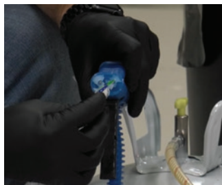
Application of petroleum jelly to spray gun
