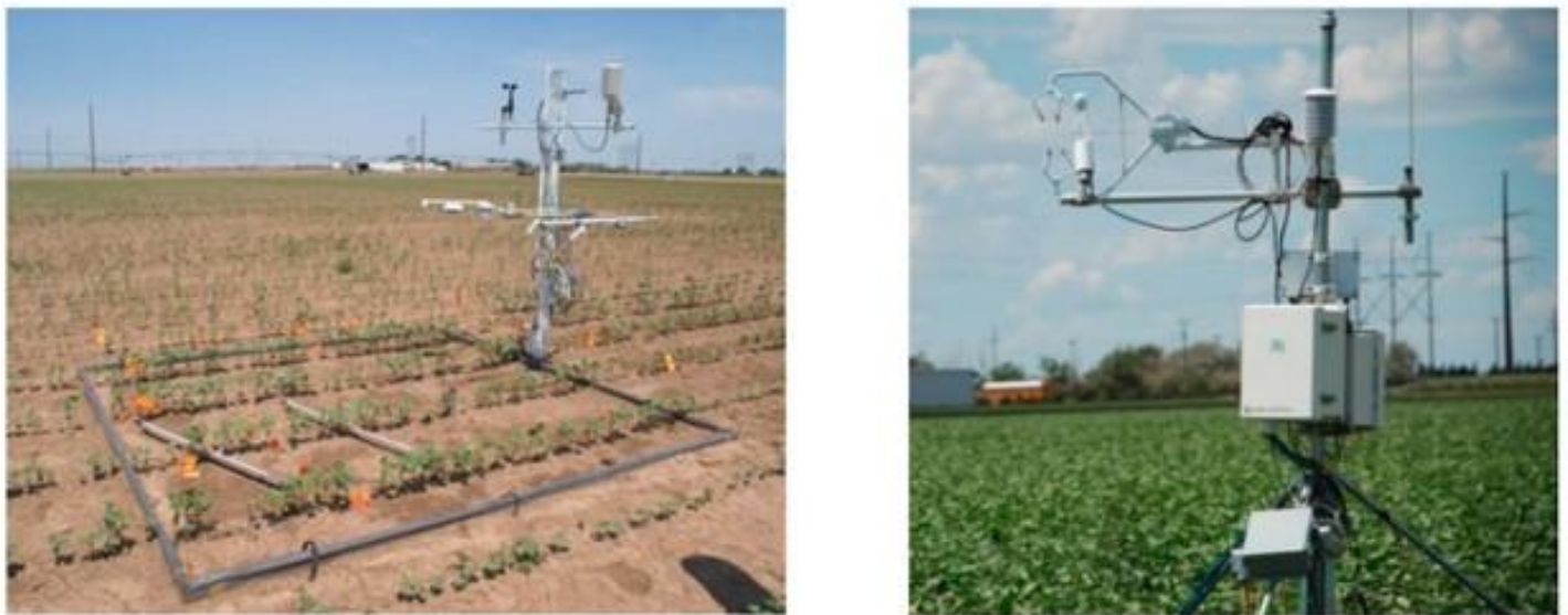
Figure 3. A flux tower is used to measure crop ET by measuring the flux of water vapor and performing calculations based on principles from the conservation of energy. Reprinted from Joy and Chavez (2021).
