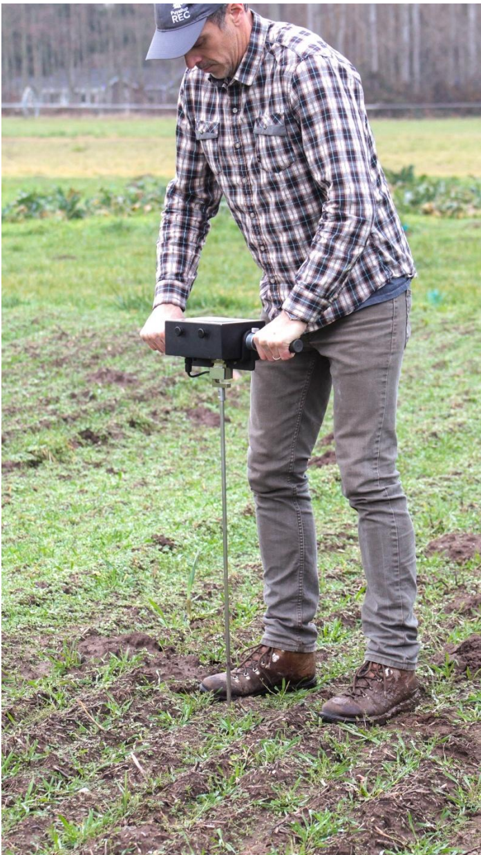
Figure 5. Methods for monitoring soil compaction include bulk density (top left photo), penetration resistance (right photo), and saturated hydraulic conductivity (bottom left photo). (Figure credit: Douglas Collins.)
