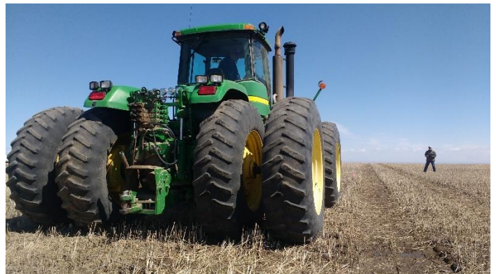
Figure 1. Heavy equipment can cause both surface and deep soil compaction. (Figure credit: Gabriel LaHue.)
