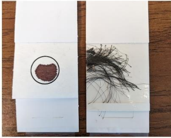
Figure 2. Two means of collecting samples for DNA testing. On the right, hair is collected and attached to the fast technology for analysis of nucleic acids (FTA) card produced by Flinders Technology Associates with follicle bulbs intact. On the left is an FTA card used for collecting blood samples. Photo credit: Allison Herrick.
