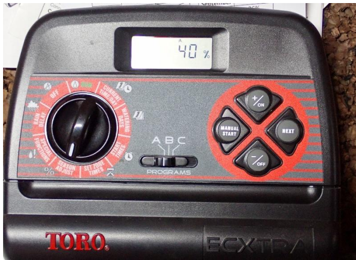
Figure 6. Automatic sprinkler controllers vary by manufacturer, but many will have a “Budget” or “Season Adjust” feature as shown here. Photo: A. McGuire.
