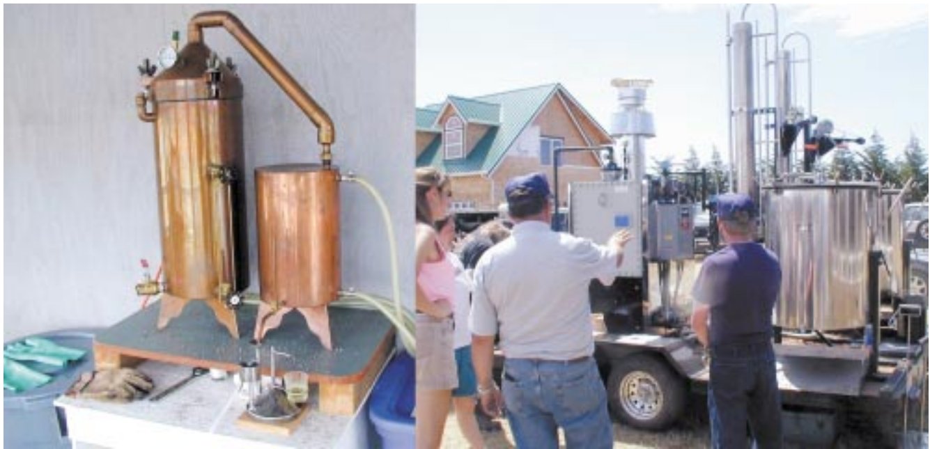
Figure 16. Left: table-top essential oil still used for small-scale distillation (also used for the trials reported in Tables 3 and 4). Right: larger, mobile commercial essential oil still.
