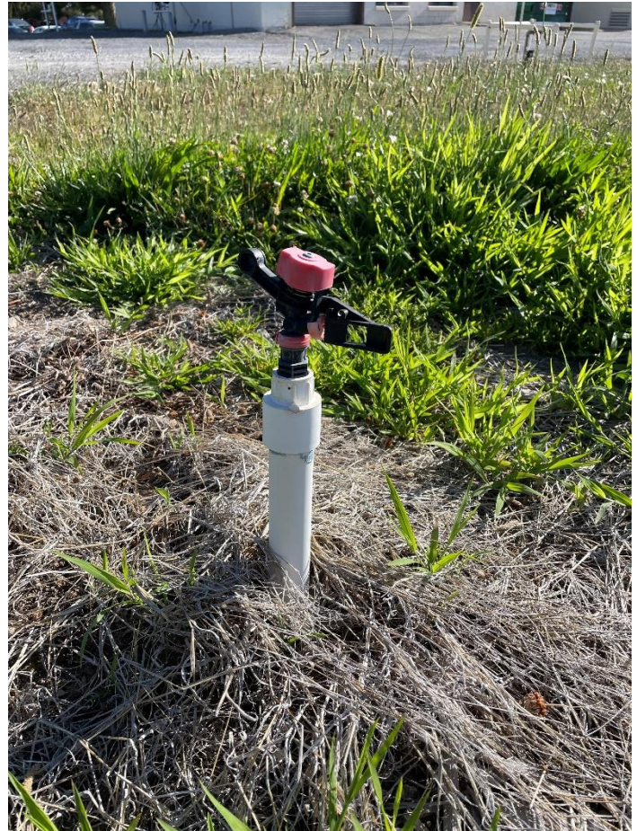
Figure 3. Impact sprinkler at Washington State University's Tree Fruit Research and Extension Center. (Photo: L.E. Flandermeier.)
