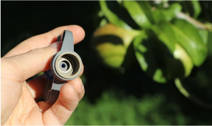
Figure 10. Flexible flow washers in flow control nozzles reduce the orifice opening and size and emit a constant flow over a wide range of pressure.
