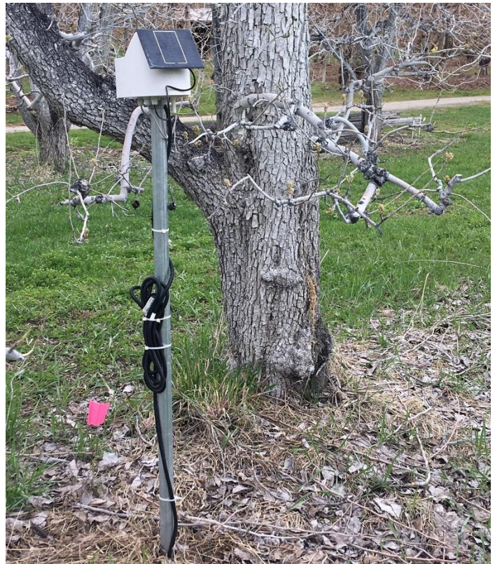
Figure 17. Telemetry for soil moisture probe installed in upgrade block.
