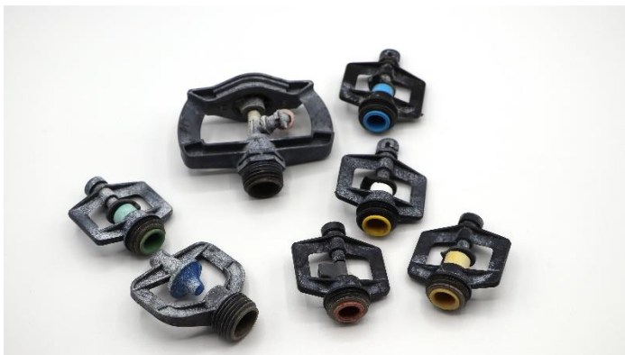
Figure 8. Multiple types of sprinkler nozzles were used in the standard block.
