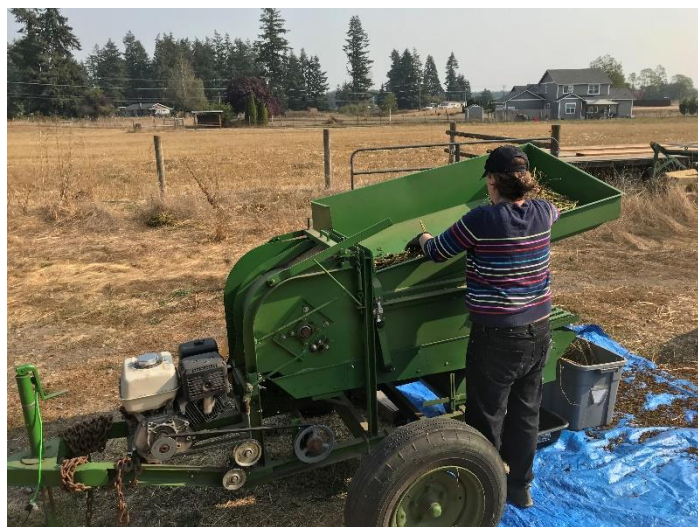
Figure 12. Swanson B1 stationary thresher. This machine has typical grain threshing adjustments, including fan speed, concave spacing, and chaffer angle. It can be used to thresh a variety of grain sizes and is effective for threshing buckwheat with minimal green matter contamination. Sheaves are fed into the threshing unit from the tray as shown here. Threshed seed deposits into a base below the unit and chaff is blown out the end to the right. Power is generated from the mounted auxiliary engine. Photo: J. O'Dea.
