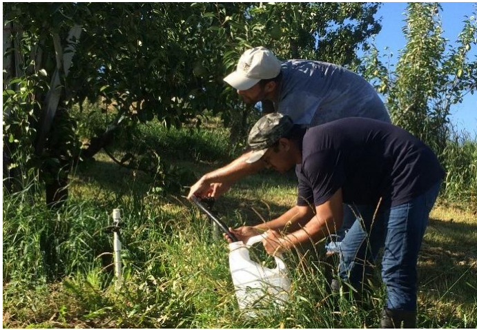
Figure 1. Graduate students diverting the flow from an irrigation sprinkler into a container for one minute in order to measure the flow rate. Photo credit: Troy Peters.
