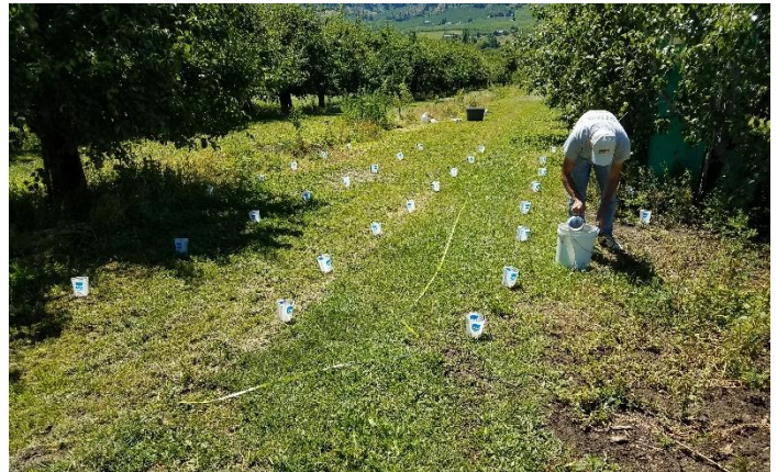
Figure 3. Place catch cans in a grid pattern with one line of cans in each tree row, one in the grass strip, and another two lines halfway between the middle of the grass strip and the tree row. Photo credit: Tianna DuPont.
