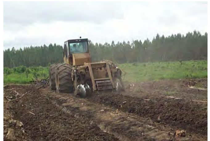
Figure 5.5. Bedding can be done at wet sites to elevate the surface soil to improve nutrition and increase soil oxygen levels. Photo: J. Espinoza.
