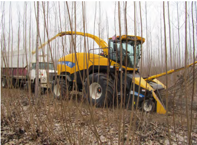
Figure 11.5. Truck positioned behind the harvester collecting biomass. Photo: S. Kar.
