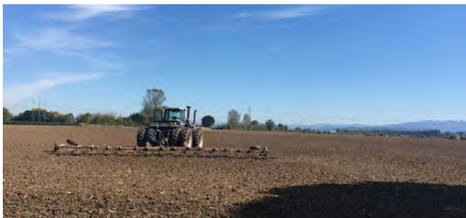
Figure 13.11. A finish disc was used to smooth the soil in preparation for a new wheat crop. Photo: R. Stonex.
