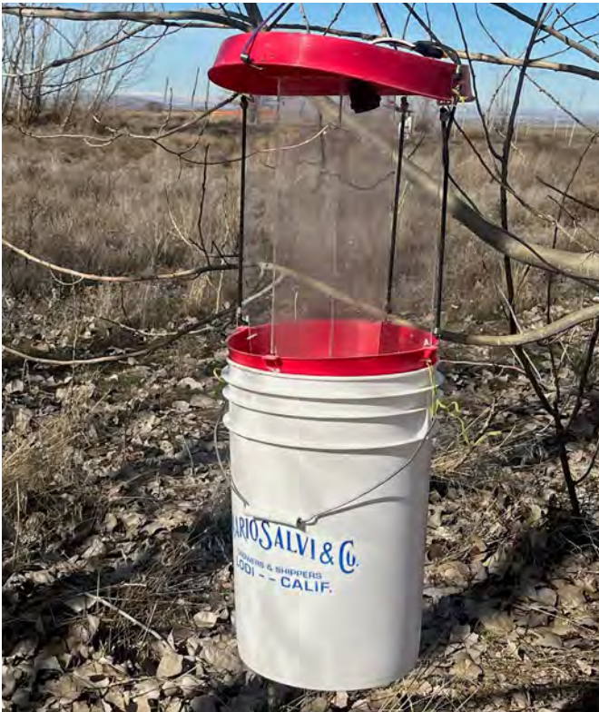
Figure 7.14. A bucket equipped with a light socket for trapping nocturnally active insects. Photo: R.A. Rodstrom.
