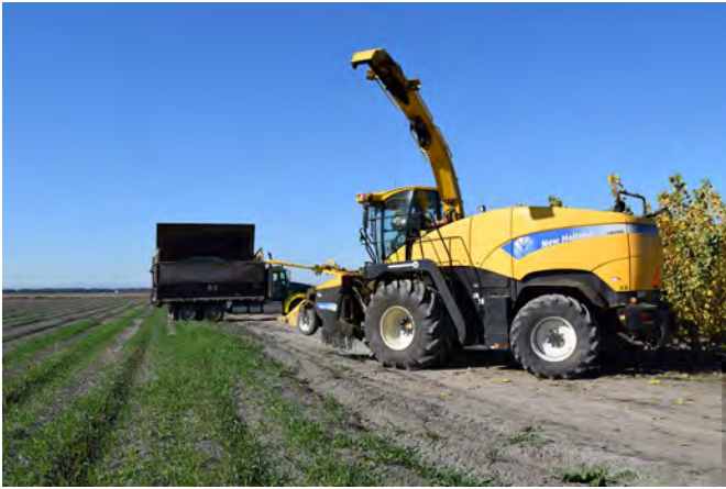
Figure 4.4. At this poplar plantation in Clarksburg, California, the headland space allows for just enough room for the harvesting equipment to make a smooth turn during harvest. Photo: N. Haider.
