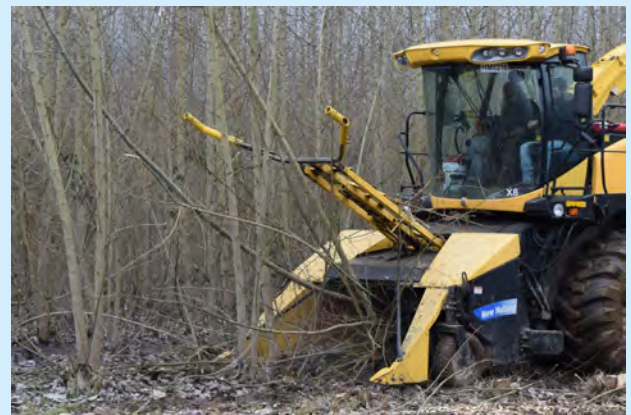
Figure 11.2. New Holland 130FB Coppice Header harvesting a row of poplars. Photo: N. Hart.
