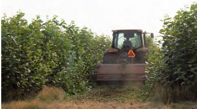
Figure 13.9. The tractor-powered Prinoth M550 is used to mulch stumps and poplar regrowth in August after a late winter harvest. Photo: P. Townsend.
