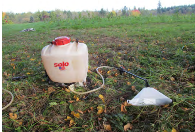
Figure 6.7. A backpack sprayer with a shield. Photo: N. Haider.
