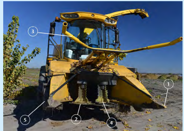
Figure 11.1. Parts of the New Holland 130FB Coppice Header. Photo: N. Haider.
