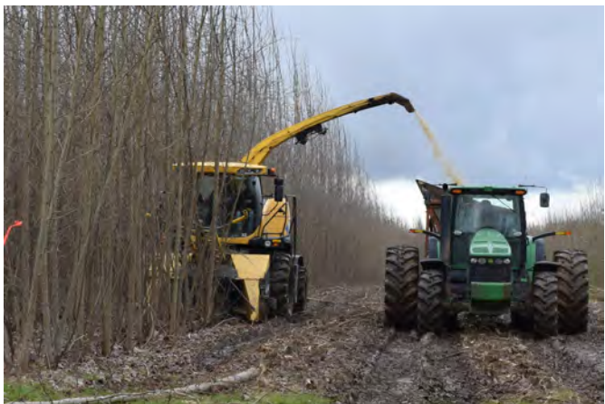
Figure 1.6. Poplar grown as a bioenergy crop is harvested using a single-pass system that cuts and chips the trees as the harvester moves down the crop row. Photo: N. Haider.
