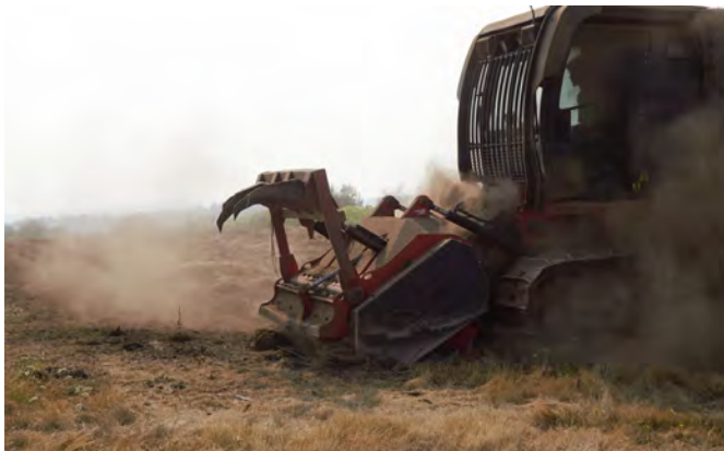
Figure 13.10. The purpose-built Raptor 800 incorporates the mulched biomass and belowground root material into the soil. Photo: P. Townsend.
