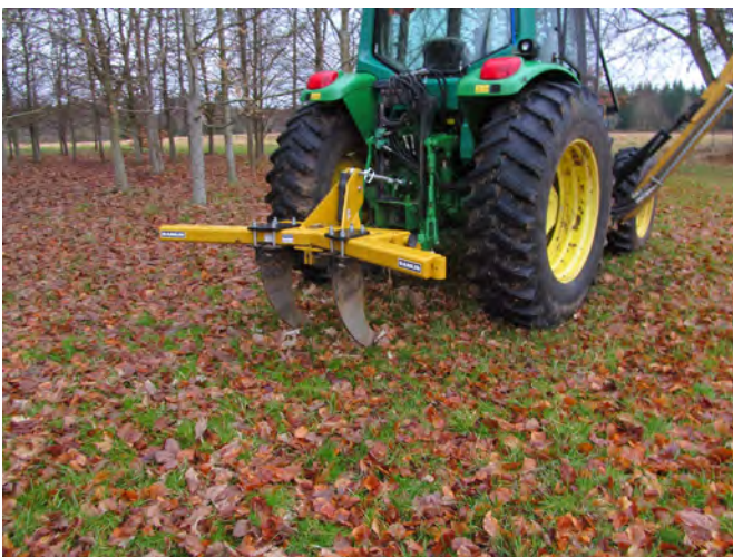
Figure 5.4. This tractor is equipped with double shanks 18 inches (46 cm) apart to create offset rows where the poplars are planted 9 inches (23 cm) off the row center. Photo: N. Haider.
