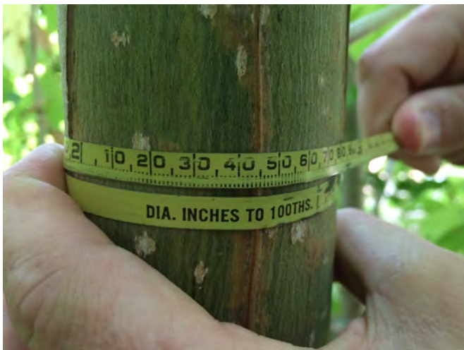
Figure 17.3. A diameter tape is used to measure DBH based on the tree's circumference. Photo: J. Espinoza.
