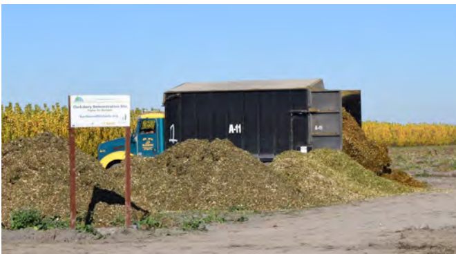
Figure 11.6. Live bottom trailer unloading wood chips. Photo: N. Haider.
