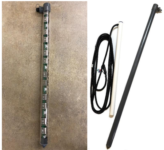
Figure 5. Capacitance probe with (left photo) and without (right photo) the plastic case. Sensors are encased and the probe is direct buried. Photo credits: Paolo Sanguaneko and Tianna DuPont.
