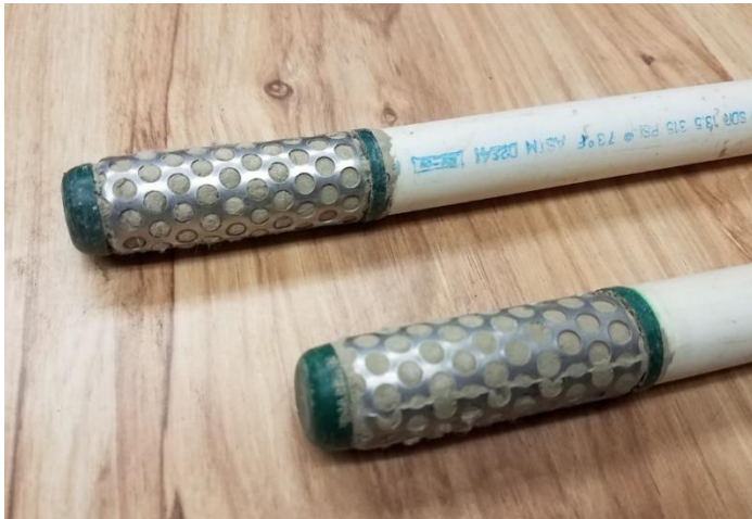
Figure 3. Granular matrix sensors (Watermark Sensors) that have been glued onto the end of PVC tubing for easier soil installation. The electrical leads are inside the tubing. Photo credit: Troy Peters.
