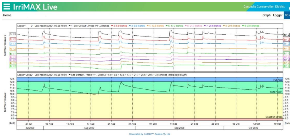
Figure 11. Example sensor output from Sentek using IrriMAX Live software. Graphic at top shows soil moisture at each sensor depth. Graphic at bottom shows the total soil moisture compared to user-designated full point (blue) and refill point (green to yellow). User can choose to display in centimeters or inches. Available with soil probes from Sentek.
