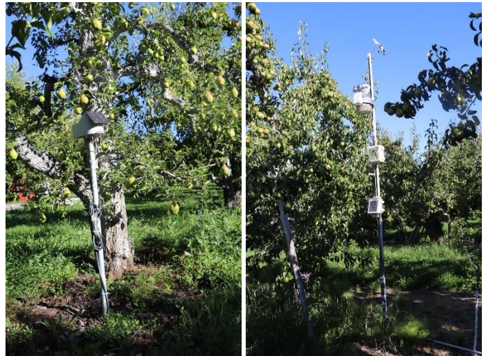
Figure 9. Telemetry systems transmit the data for off-site access. Photo credits: Tianna DuPont.
