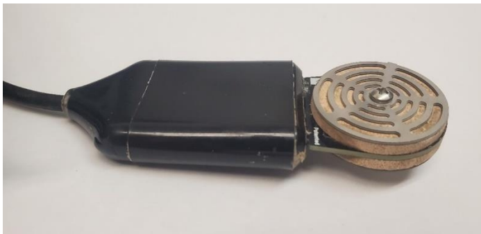
Figure 4. A TEROS 21 soil water potential sensor manufactured by METER Group (Pullman, WA). Photo credit: Troy Peters.
