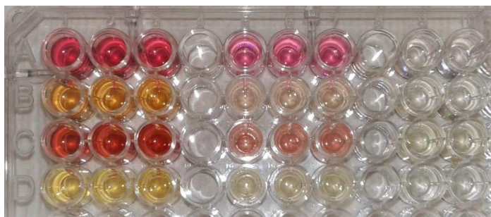
Figure 1. Porter assay showing juices of ‘F1-hybrid crab’ in row A, ‘IRM’ in row B, ‘Dabinette’ in row C, and ‘Golden Delicious’ in row D. Left to right indicates assay with HCl, assay without HCl (a blank), and the final blank. The reddish color indicates a high, low, or zero level of tannin as anthocyanidin. The absence of HCl in the blank or middle section implies less background flavan-3-ols which convert to anthocyanidins, the final reaction product. Photo by D.S. Mattinson.
