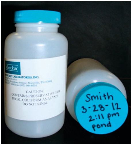
Figure. 2 Sampling bottle properly labeled with name, date, time, and type of water source. (Photo by: Annette Wszelaki.)
