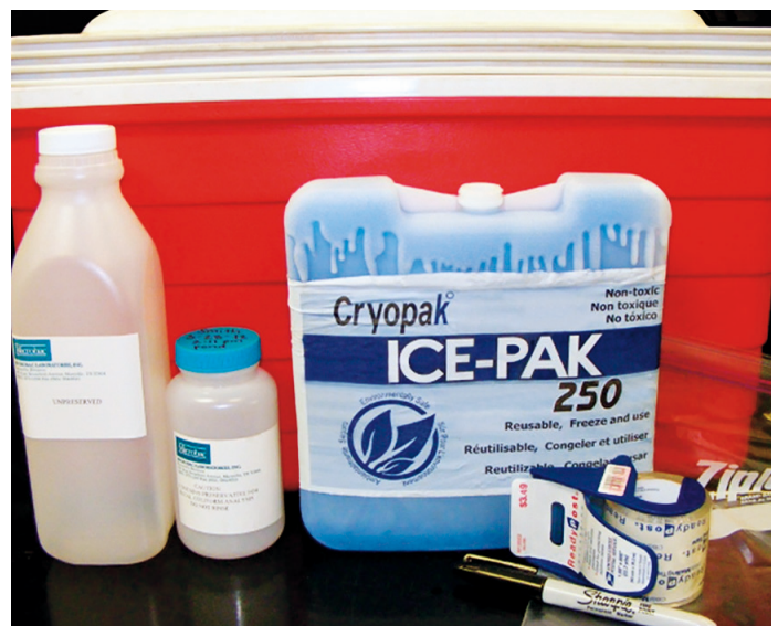
Figure 1. Water sampling supplies: cooler, ice or ice packs, sampling bottles, marker, Ziploc bag, tape. (Photo by: Annette Wszelaki.)
