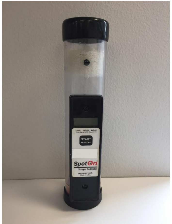
Figure 9. Example of a low volume flow meter. This model is accurate for volumes under 1 GPM, which is appropriate for most nozzle selections. Photo by Gwen-Alyn Hoheisel, WSU.
