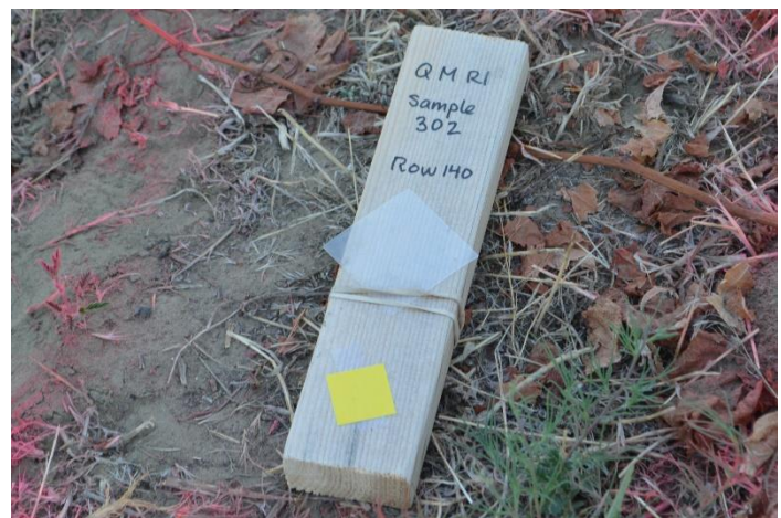
Figure 11. A small wooden block with WSP taped to it placed on the ground one to three rows downwind from the sprayer to provide a visual assessment of how much spray is lost to the ground. Photo by Margaret McCoy, WSU.
