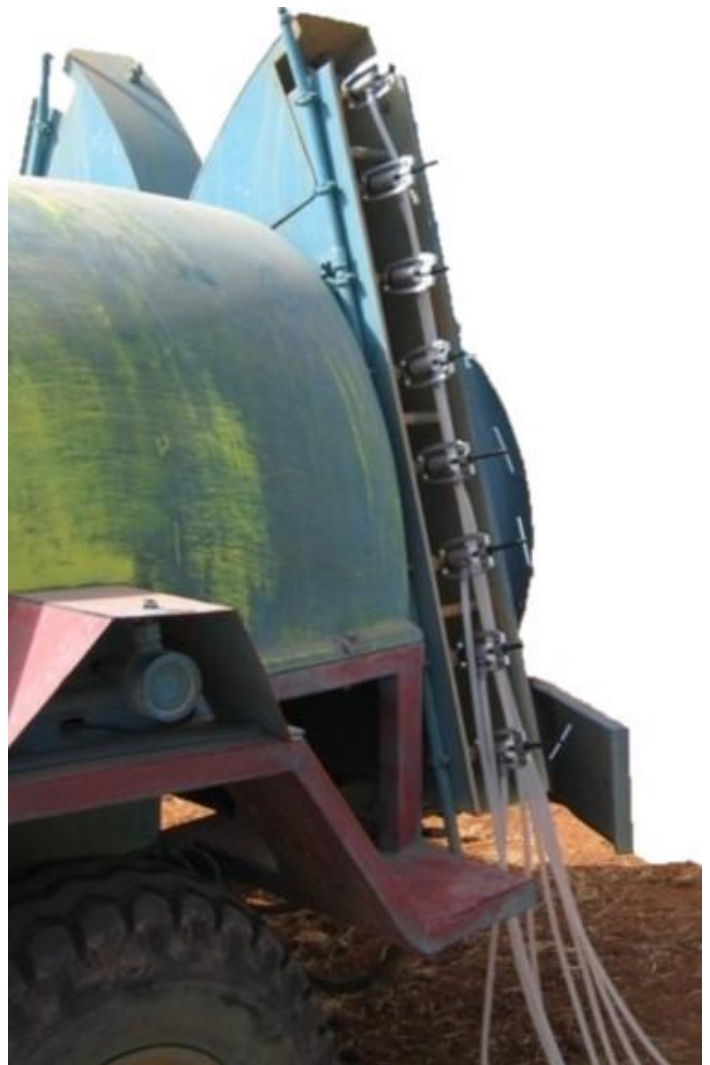
Figure 10. AAMS nozzle clamps connected to a sprayer. Output will be measured from each tube coming from the clamp. Photo by Gwen-Alyn Hoheisel, WSU.
