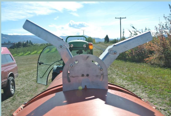
Figure 4. Longer deflectors help guide the air to make it even on both sides. Deflectors are often set incorrectly by using similar positions on the right and left. If the fan is rotating clockwise, the right arm of the deflector (looking from the back of the sprayer) should be more vertical since air is already being pushed down, while the left side should be more horizontal to the ground to adjust for the air that is being pushed up by the fan. Photo by Steve Castagnoli, OSU.
