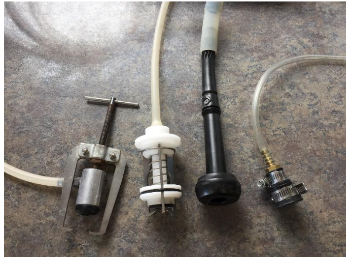
Figure 8. Nozzle clamps to cover the nozzle and measure water output. This image shows both purchased and homemade options. From left to right are: AAMS clamp, Herbst clamp, homemade clamp from cow milking parts, and homemade clamp from plumbing parts. Photo by Gwen-Alyn Hoheisel, WSU.
