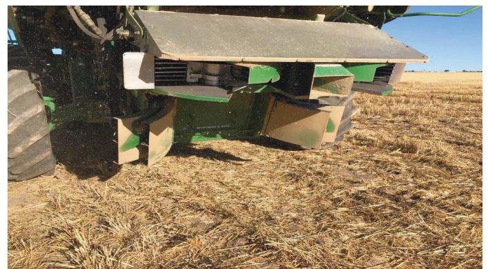
Figure 4. Integrated Harrington Seed Destructor mounted at the rear of the combine.
