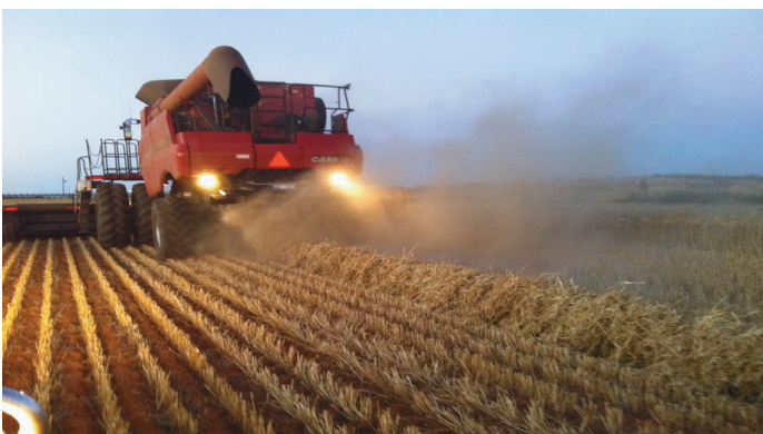
Figure 2. Narrow windrows formed with chaff chute on rear of combine (left) are burned (right) in the fall under cooler and more humid conditions.
