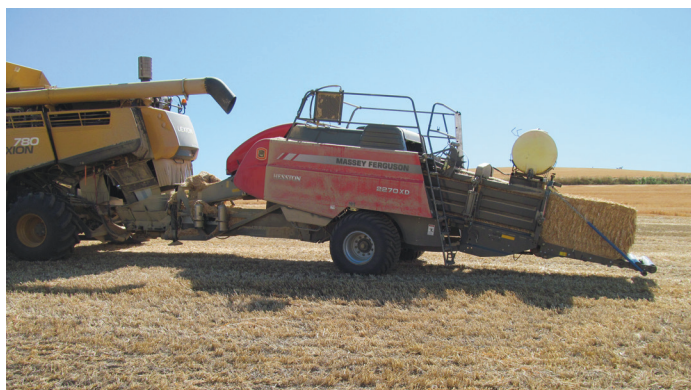
Figure 3. With the bale direct system, straw and chaff (containing weed seed) are baled together directly behind the combine.
