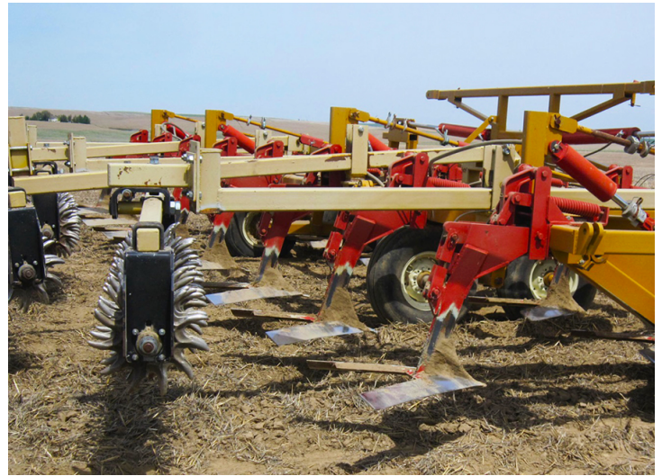
Figure 3. Undercutter implements have blades on two ranks to allow easy passage through high levels of residue without plugging. This unit is equipped with an attached skew treader to size soil clods. The angle of the skew treader attachment can be adjusted to achieve the desired size of surface soil clods. Photo by W.F. Schillinger.
