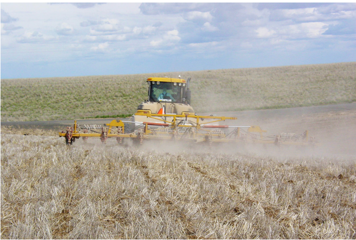
Figure 2. The undercutter's narrow-pitched and overlapping 32-inch-wide V blades slice beneath the soil at a depth of five inches to completely sever capillary channels and halt the upward movement of liquid water to retain seed-zone water in summer fallow for late-summer planting of winter wheat. Most of the winter wheat residue from the previous crop is retained on the surface to control wind erosion. Photo by W.F. Schillinger.
