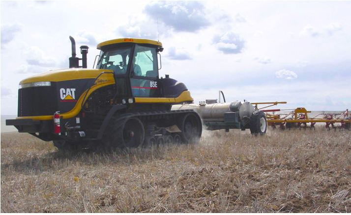
Figure 1. A 375-horsepower crawler tractor pulls a 1,000-gallon tank cart filled with aqua NH 3 -N and a 32-foot-wide undercutter implement during primary spring tillage plus nitrogen and sulfur fertilizer injection in April. Photo by W.F. Schillinger.
