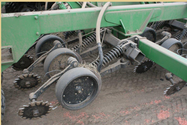
Figure 4. Exapta (or Thompson) closing wheel (spiked wheels on far left). Photo: Guy Swanson.
