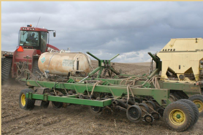
Figure 3. Odberg's drill and fertilizer delivery system. Photo: Guy Swanson.
