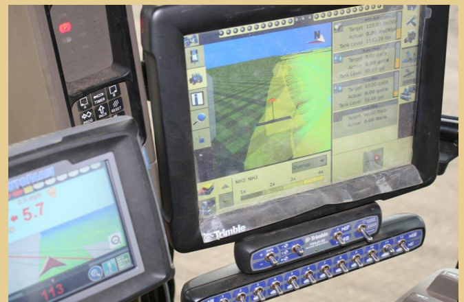
Figure 5. Trimble FMX controller (screen on the right) which can independently control the rate of up to four products. Raven Envizo Pro (smaller screen on the left) carries out auto-steer and provides guidance. Photo: Guy Swanson.
