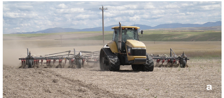
Figure 3. A 10-inch sweep on an 8-inch shank spacing was run two inches deep to sever weeds not fully controlled by glyphosate application.
