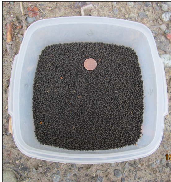
Figure 3. Pellets of heat-dried biosolids. (Photo by Craig Cogger, WSU Extension)
