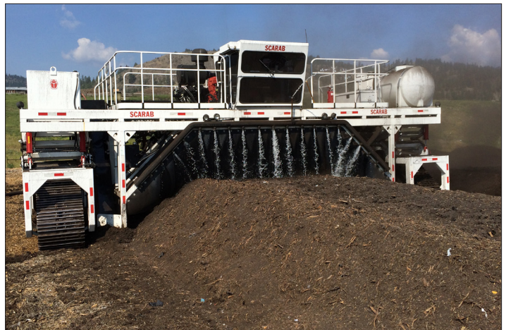
Figure 4. Making biosolids-yard debris compost using a turned windrow system, Kelowna, BC. (Photo courtesy of Gordon Light, City of Kelowna, BC)
