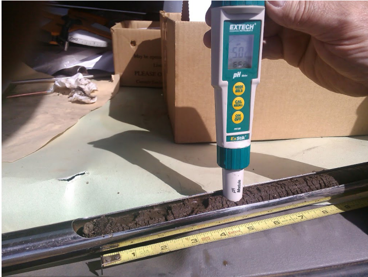
Figure 1. Example of checking soil core at 1-inch increments using a soil pH meter. Photo: Paul Carter.
