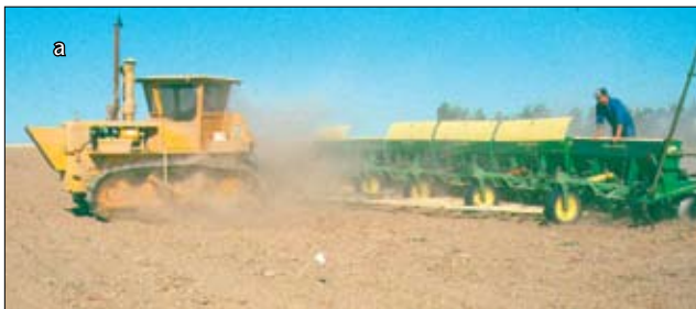
Fig. 16a. Development of the deep-furrow split-packer John Deere HZ drill in the mid-1960s was a major advancement for winter wheat–summer fallow farming because seed could be placed up to seven inches below the surface into moist soil. This allowed farmers to establish wheat early (late August–early September) for optimum grain yield potential. Fig. 16b. Deep furrows spaced 16 inches apart help minimize the soil cover over the seed, but winter wheat seedlings still have to elongate through 4 to 6 inches of soil to reach the surface. The drags behind the drill are sometimes used to help stabilize the furrow and reduce the thickness of soil covering the seed. Photos by W.F. Schillinger.
