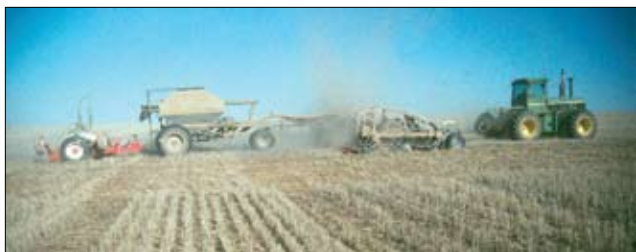
Fig. 18. A modern Flexi-coil no-till drill delivers seed and fertilizer in one pass through the field. This 33-foot-wide drill has an attached tank cart that carries seed in one section and granular starter fertilizer in the other section. Aqua NH 3 -N, carried in the 1000-gallon tank at the end, is pumped forward and delivered slightly to the side of and below the seed. Photo by W.F. Schillinger.
