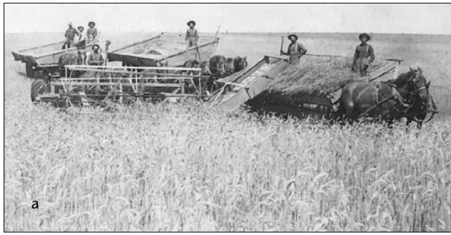
Fig. 5a. Cutting and loading wheat in the field with a header into a header wagon for transport to a threshing site. The header is equipped with a reel that lays the wheat stalks across a reciprocating sickle bar for cutting standing grain and onto a canvas platform for elevating into the wagon. It is ground-driven, cuts a swath 12- to 20-feet wide and is pushed from the rear by six horses. Courtesy, Terry Olson family, Ritzville, Washington.
