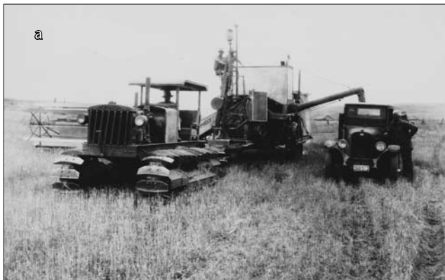
Fig.14a. This farmer in 1930 was an early convert to bulk grain harvesting. Handling grain in bulk instead of sacks dramatically reduced manpower requirements and heavy labor. An early model 30-horsepower crawler pulls the gas-powered combine. Northwest Museum of Arts & Culture, Spokane, Washington. L89-35. Fig. 14b. Unloading bulk wheat at a grain elevator during the 1930s. The front of the truck was raised by a mechanical lift. Washington State Historical Society, Tacoma, Washington.
