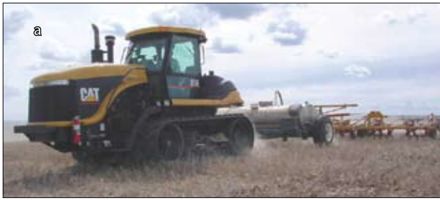
Fig. 19a. A modern 375-horsepower Caterpillar 85E crawler tractor pulls a 1000-gallon tank filled with aqua NH 3 -N, and a Haybuster undercutter during primary spring tillage plus N fertilizer injection near Lind, Washington. The 32-foot-wide implement is operated at 6 mph and covers about 185 acres per day. The tank needs to be refilled with aqua NH 3 -N every hour. Fig. 19b. The wide, narrow pitch, and overlapping V-blades on the undercutter implement slice below the surface with little soil lifting or disturbance of surface residue, but completely sever soil capillary continuity and halt upward movement of liquid water to maintain seed-zone moisture in summer fallow. Note the standing stubble that is much more effective than flattened stubble for wind erosion control. This represents the best technology currently available for profitable and environmentally sound winter wheat–summer fallow farming in the low-precipitation zone of the Pacific Northwest. Photos by W.F. Schillinger.
