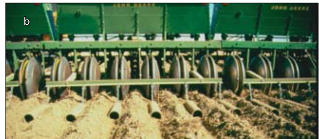
Fig. 16a. Development of the deep-furrow split-packer John Deere HZ drill in the mid-1960s was a major advancement for winter wheat–summer fallow farming because seed could be placed up to seven inches below the surface into moist soil. This allowed farmers to establish wheat early (late August–early September) for optimum grain yield potential. Fig. 16b. Deep furrows spaced 16 inches apart help minimize the soil cover over the seed, but winter wheat seedlings still have to elongate through 4 to 6 inches of soil to reach the surface. The drags behind the drill are sometimes used to help stabilize the furrow and reduce the thickness of soil covering the seed. Photos by W.F. Schillinger.
