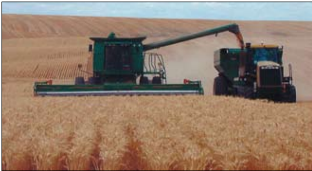
Fig. 20. A new John Deere 9760 level-land combine with 30-ft header unloads wheat on the go near Ritzville, Washington, in July 2006. The grain yield of soft white winter wheat in this field averaged 48 bu/acre. The combine operated at a speed of 5 mph and harvested 18 acres per hour. Farm machinery costs have skyrocketed in recent decades. This combine was rented from an equipment dealer for $150 per separator per hour. The price of a new machine is $250,000. Photo by Derek Schafer, Ritzville, Washington.
