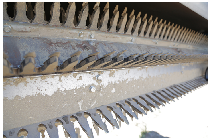
Figure 9. Fingers in the header, which strips the wheat head from the stalk, need to be replaced periodically. The Jurises have found overall maintenance costs to be similar for a traditional header and a stripper header. Photo: Matt Ziegler.
