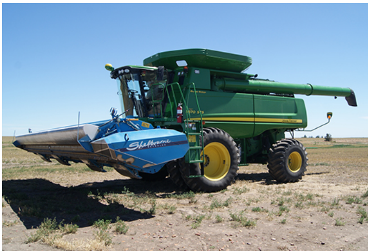
Figure 7. The Jurises’ stripper header, mounted on their combine. Photo: Hilary Davis.
