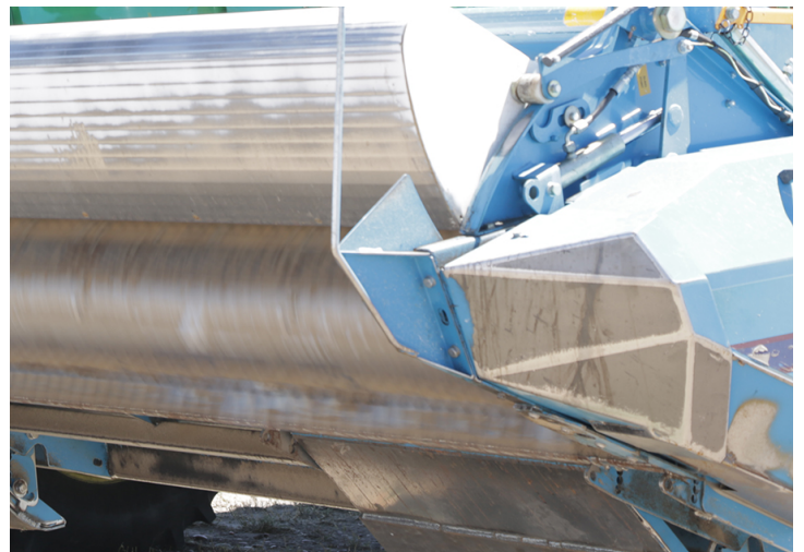
Figure 8. Skid plates on the bottom of the stripper header help protect it from damage from rocks. Photo: Matt Ziegler.
