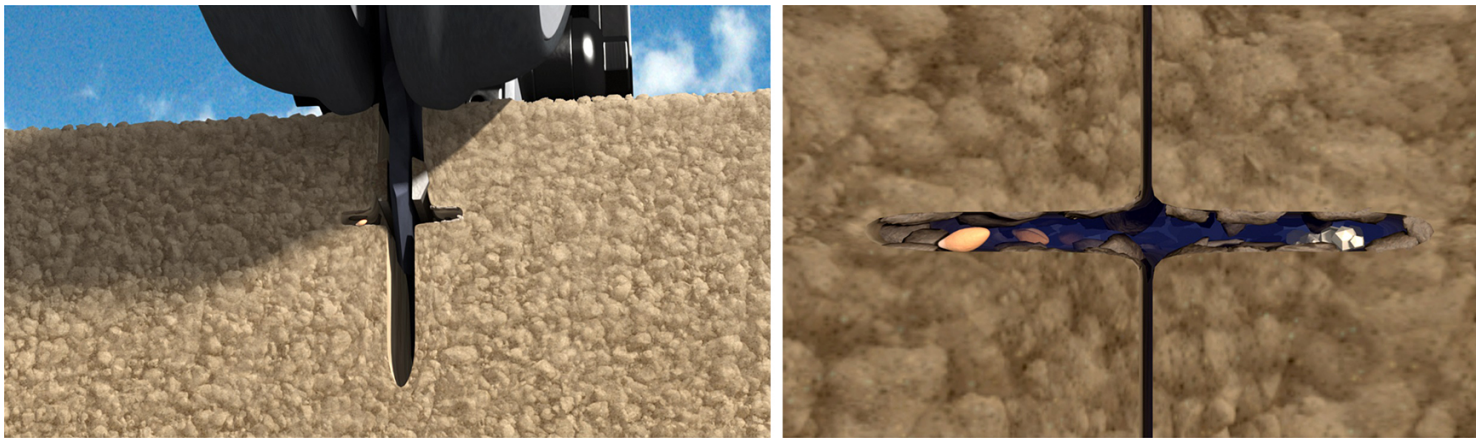
Figure 6. Rendering of a cross slot drill, showing the narrow hoe opener and disc blade (L). The seed and fertilizer are placed in the horizontal slot (R). Graphics: Baker No-Tillage Limited.
