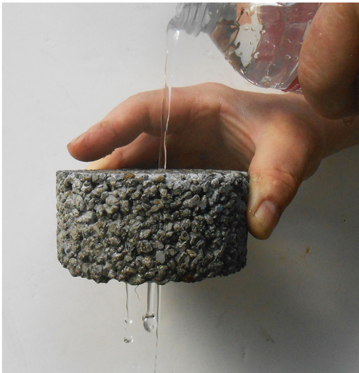
Figure 19. Permeable pavers and porous concrete allow water to soak through. Photo by Kathleen Chase.
