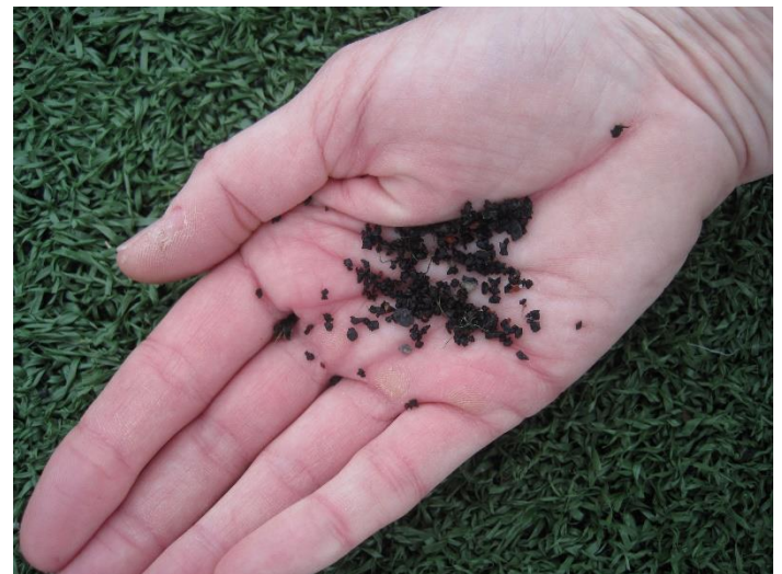
Figure 3. Crumb rubber is a more finely ground version of rubber mulch. Photo: L. Chalker-Scott.
