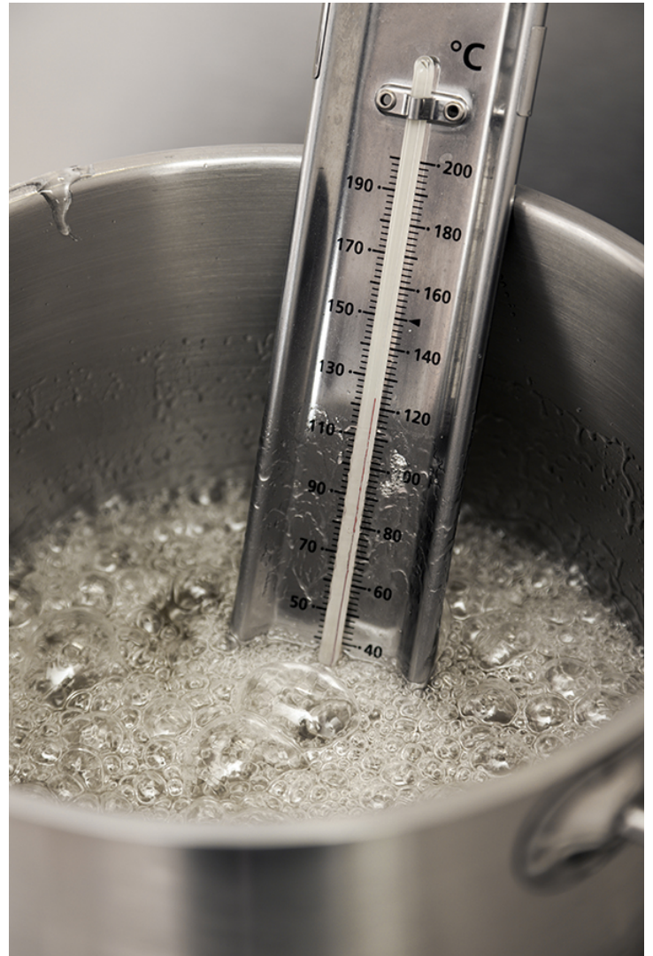
To measure the temperature of cooked product, use a candy or jelly thermometer.
