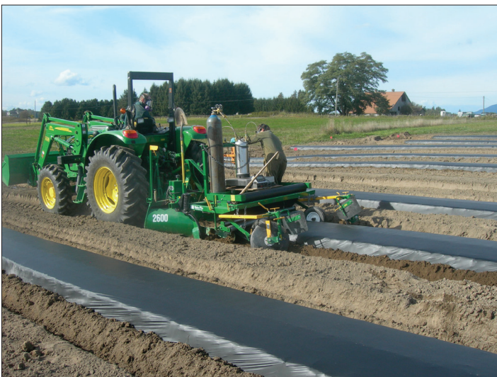
Figure 3. Bed fumigation prior to planting raspberry. Planting beds are formed, fumigated, and covered with an impermeable tarp in a single operation.
