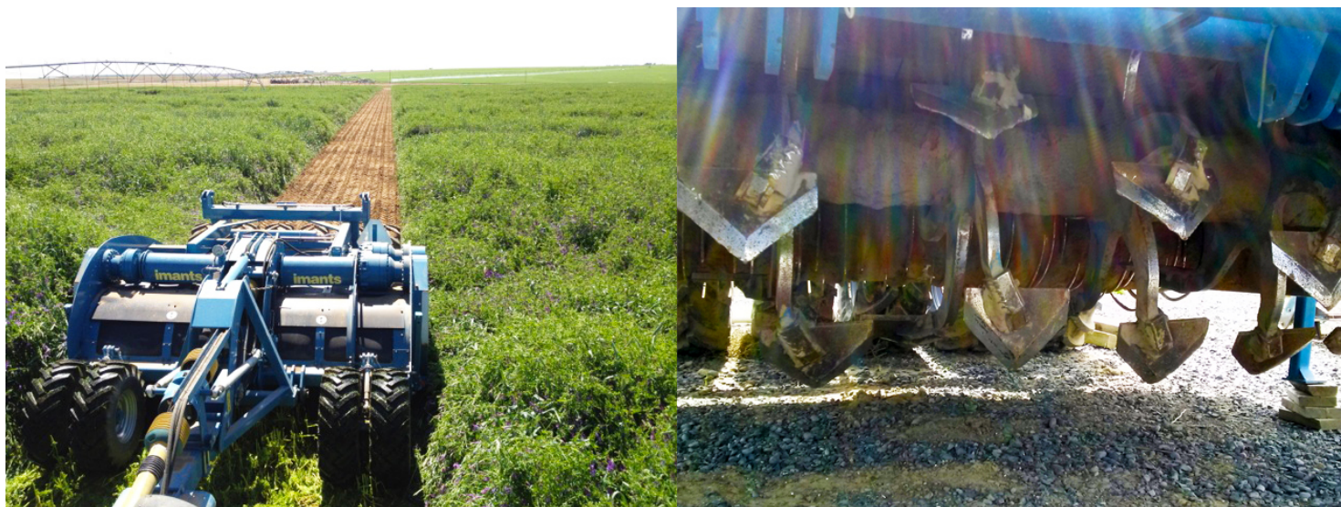
Figure 10.3. Using a spader (left) to incorporate a vetch-triticale cover crop and (right) a close-up view of the spades attached to a central rotor. (Photos by Brad Bailie (left) and Louise Lorent, WSU (right).)
