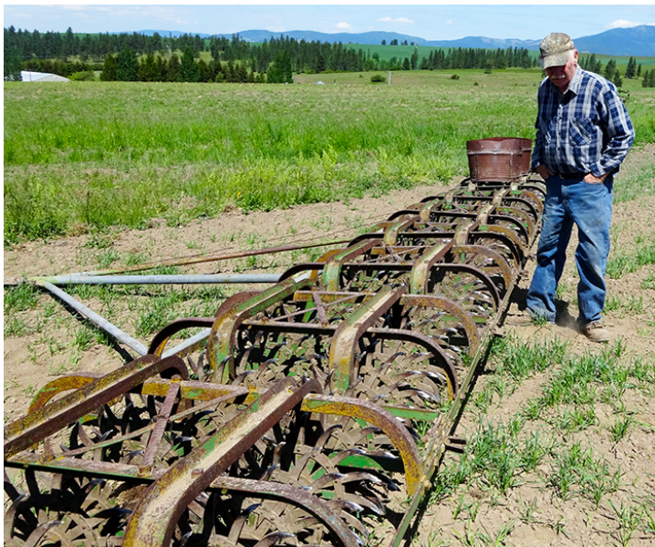
Figure 7.2. Ted Lacy's 50-ft rotary hoe consists of several units joined together. (Photo by Diana Roberts, WSU Extension.)
