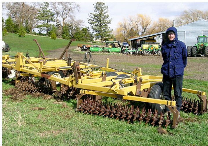
Figure 6.2. David Ostheller with a skew treader that he uses as a rotary harrow for weed management prior to planting. The angle of the implement can be adjusted to increase or decrease the aggressiveness of its action. (Photo by Diana Roberts, WSU Extension.)
