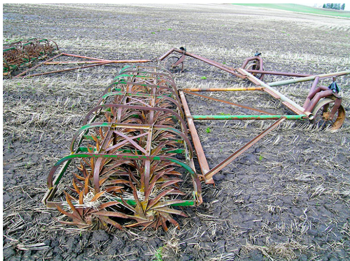
Figure 6.3. David Ostheller has adapted several sections of rotary hoe to make the implement 50 ft wide for weed management both prior to seeding and in-crop. (Photo by Diana Roberts, WSU Extension.)
