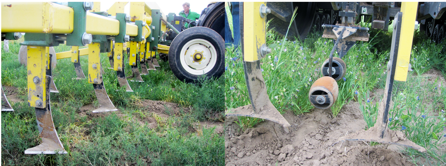
Figure 1.5. Eric Nelson’s Acura Trak (a) in-row tillage tool and (b) guidance system. (Photos by Diana Roberts, WSU Extension.)
