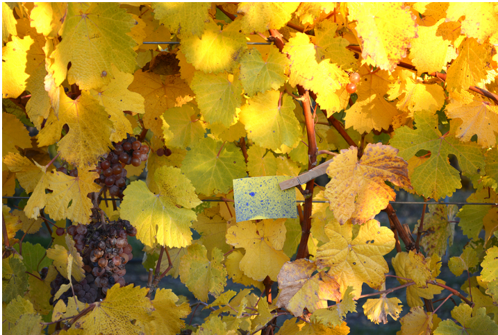
Figure 6. The deposition of a pesticide can be assessed using food-grade fluorescent dyes or water-sensitive card, as shown here. Cards should be placed in the specific areas of the canopy you are interested in assessing. When designing an experiment, each treatment replicate should have the same distribution of spray cards. For general spray assessment purposes, most cards should be placed within the fruit zone, with the water-sensitive side of the card facing outward to the vineyard row. Ideally, cards should be placed vertically in the middle of the fruit zone. Photo by Hemant Gohil.
